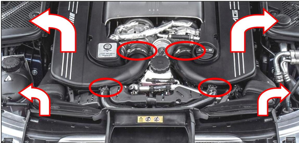
4. The sensors are located underneath an engine wiring harness, which is secured to a series of plastic covers above it, and this assembly is attached to the engine with a number of bolts and plastic barbed fasteners. This assembly must be released from the engine and allowed to slide forward about 5"-6", in order to provide access to the sensors underneath.
