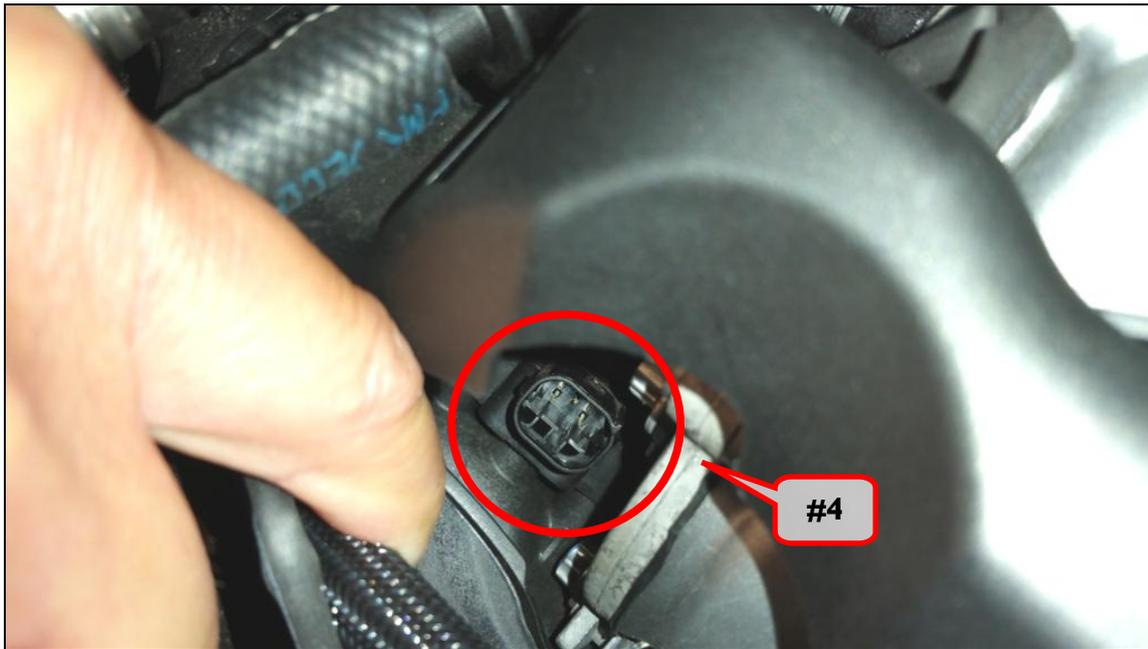
11. Study the locking system on the new DINANTronics connectors until you are familiar with how the two connector halves are released. Some locks will require the use of a small flat blade screwdriver to release the tang.
