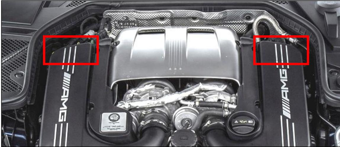
3. Release the 4 clamps indicated below, and remove both airbox assemblies from the car by pulling upwards. Also release the locking tabs and remove both intake ducts from the car.
