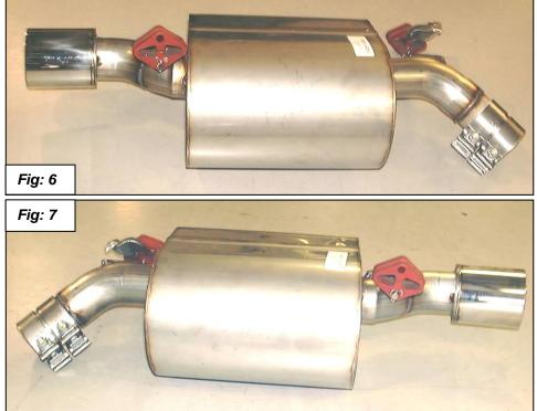
9. Install each muffler by sliding the clamps over the ends of the pipes. Attach the hangers to
