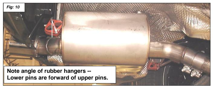
Visually inspect the muffler. Check for at least ½" clearance in all areas. Make sure the polished tips are centered in the bumper cutouts. See figure 11.
