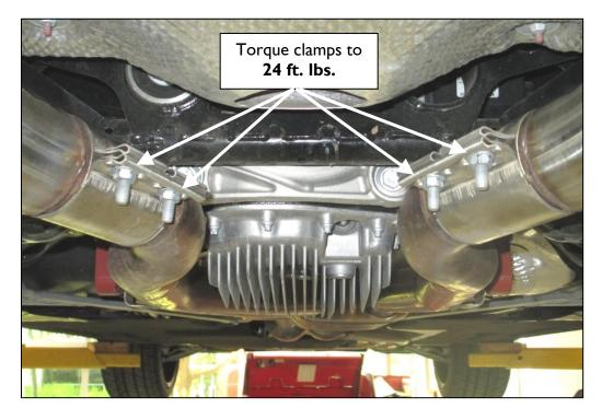
Check the exhaust tips for proper bumper clearance and proper alignment using Figures 3
