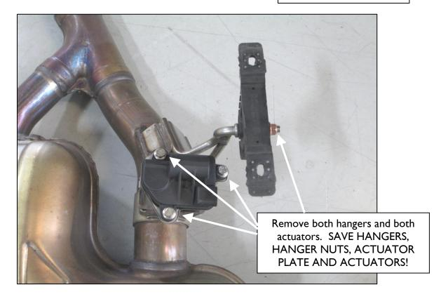
6. Install both stock hangers onto DINAN muffler using the stock hanger nut that was saved from removal.
