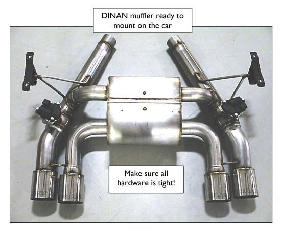
8. Place exhaust clamps provided in the hardware kit onto the ends of the stock exhaust pipes. With DINAN exhaust secured on a jack or stand, put the muffler in place. When mounting the muffler it should be held with the tips up near the bumper and the muffler pushed forward against the ends of the stock pipes.
