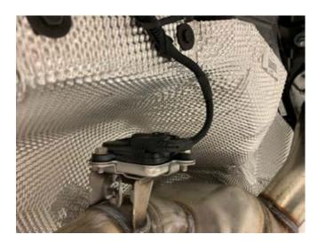
3) Unbolt the exhaust hangers and remove the stock muffler.
