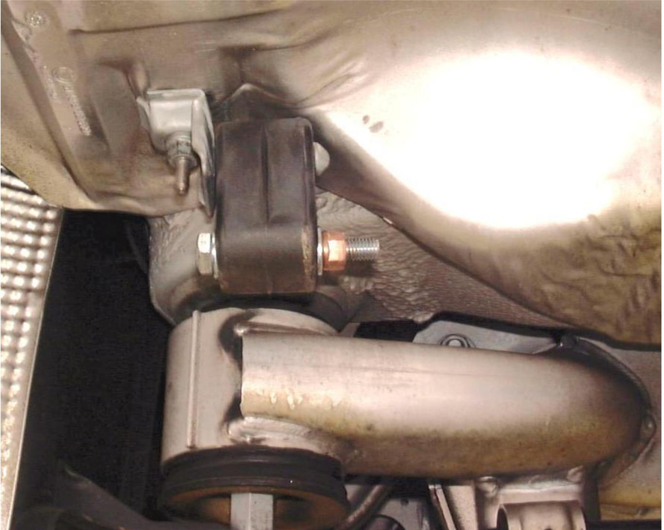
5. Deburr the inside of the stock exhaust tube on the car and clean the outside surface to ensure a good seal.
