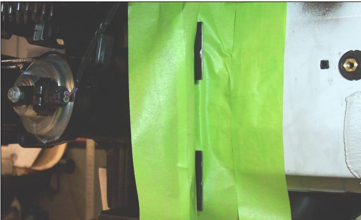
59. Reinstall the headlight assy by first starting all of the screws then tightening them with the assy positioned just like it was.
