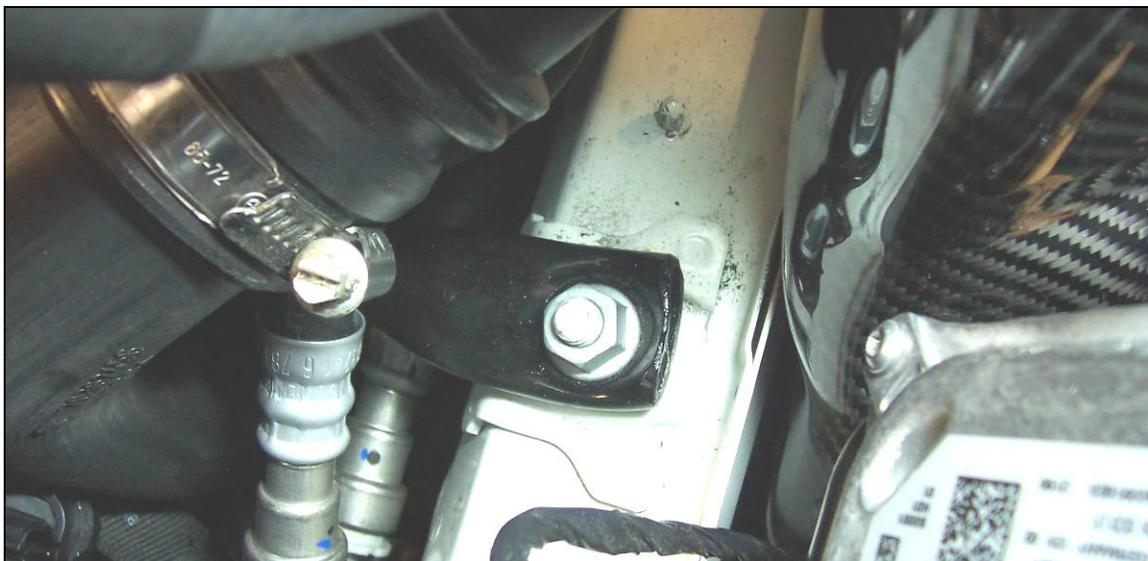
29. Unbolt the brace and carefully pull it up and outward as far as it will easily go.
