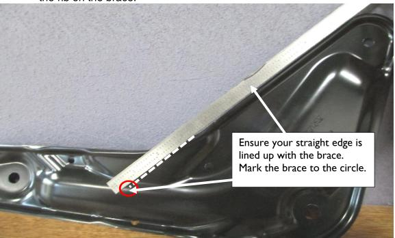
22. Now draw a line from your first mark, along the rib to just 1/4" beyond the hole where the rib starts to go back to the outer edge.
