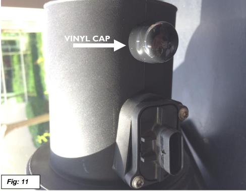
17. Install Dinan Air Filter onto the Dinan Airbox Lid/MAF. Make sure the MAF ridge is properly seated in the air filter groove. Don't tighten clamp yet. See Figures 12&13.
