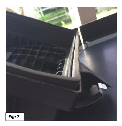
10. Remove the 4 clips from the lower airbox and install the 4 smaller clips supplied in the hardware kit. See Figure 8.
