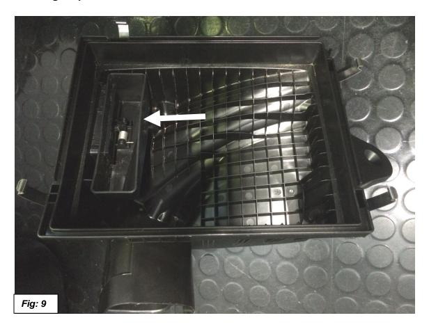
12. Remove the snow valve from the inside of the airbox by pinching the clips on the outside. See Figures 10 & 11.
