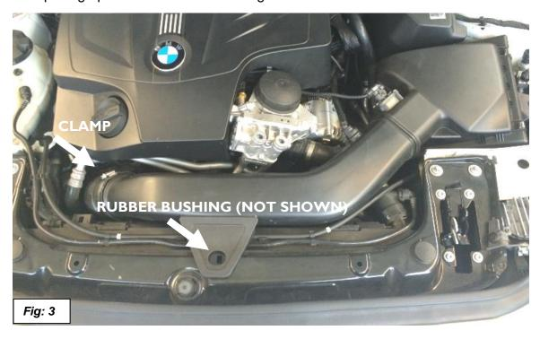
6. Remove lower airbox by gently lifting up. Remove filter. See Figure 4.
