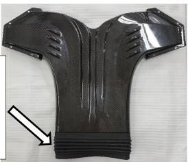
5) To install the main snorkel, slide the boot over the scoop. Make sure the boot fully surrounds the front inlet and snorkel. Check the underside fitment as an improper seal will affect performance.
