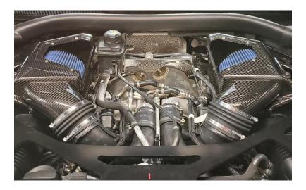
4) You can now install the Dinan Main Snorkel. Before installing, seat the main rubber boot onto the bottom of the snorkel.
