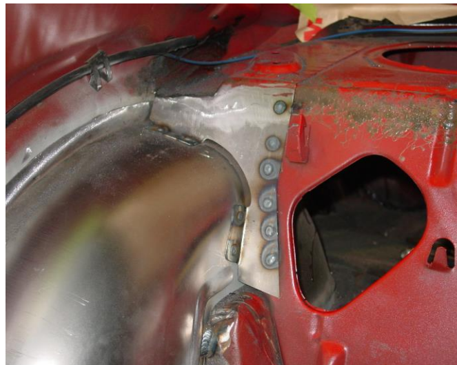
Figure 22 - Seat Back Bracket Installed
