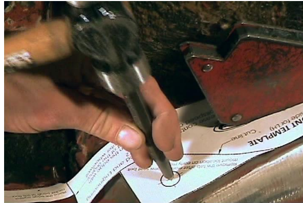
Figure 3 - Inner Wheelwell Front Template with Tab
