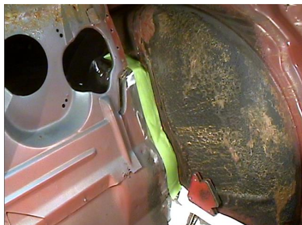
Figure 6 - Cut Line Extension Using 2" Tape
