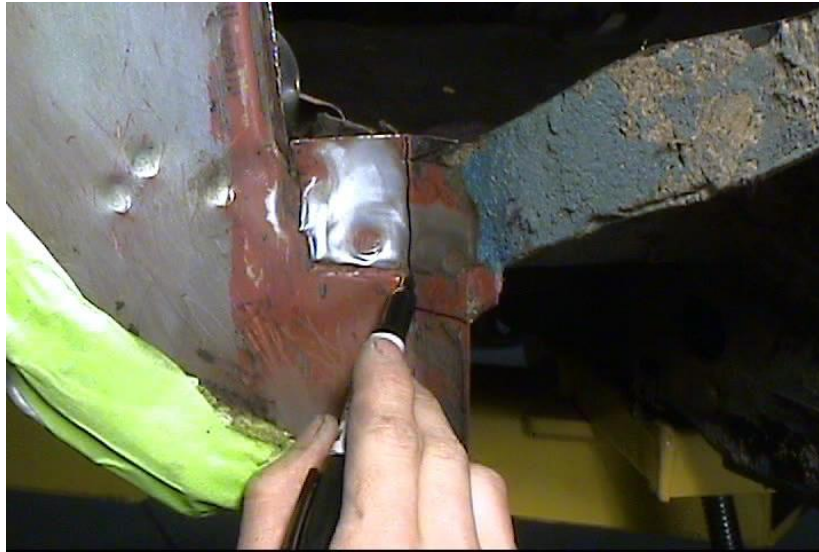
Figure 7 - Marking Tab for Removal
