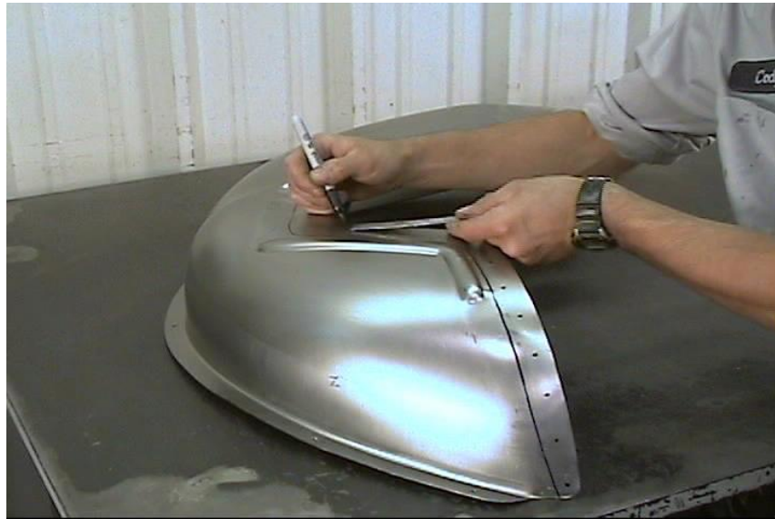
Figure 16 - Mark Tub Mounting Surfaces
