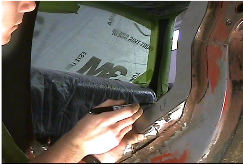
Figure 10 - Front Flange Alignment
