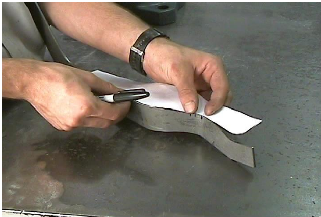
Figure 11 - Front Template Bend Profile
