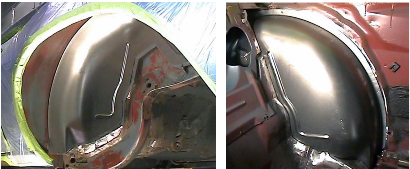
Figure 15 - Test Fit Detroit Speed Mini-Tub
