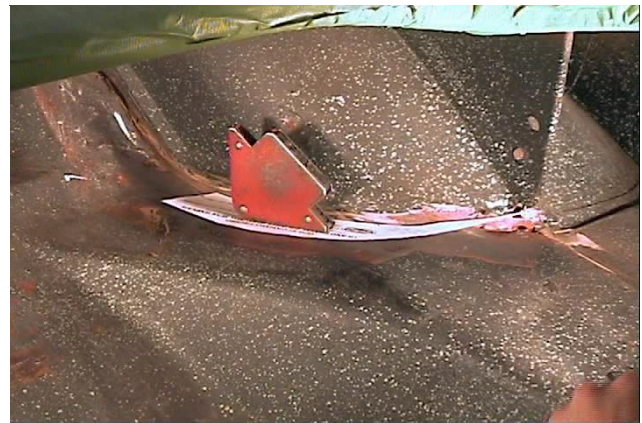
Figure 5 - Inner Wheelwell Rear Template
