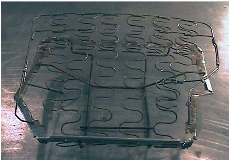
Figure 24 – Narrowed Rear Seat Frame
