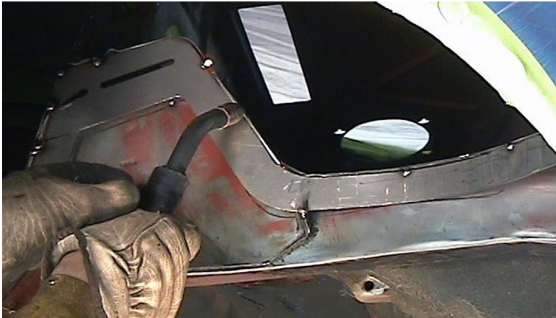
Figure 14 - Tack Weld Tub Flanges
