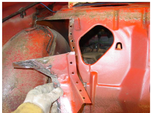
Figure 2 – Seat Support Removed
