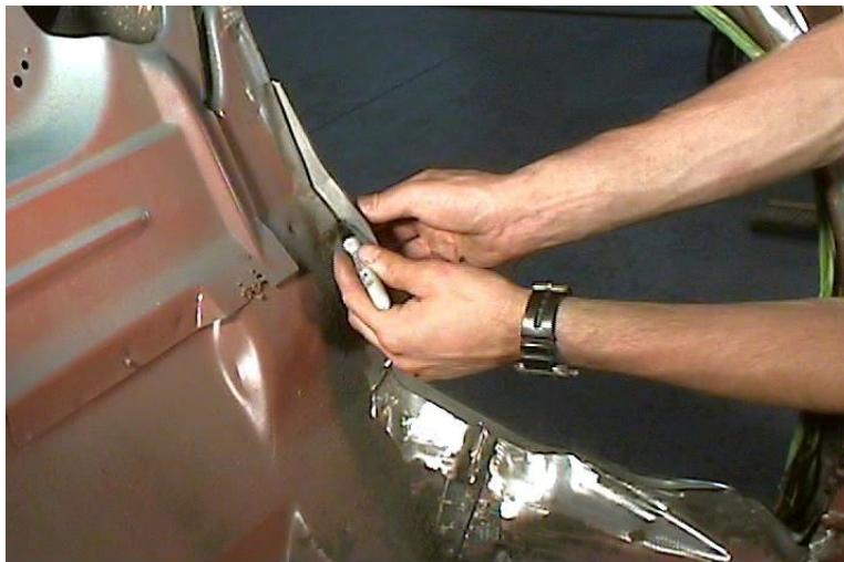
Figure 13 - Marking Front Template to Floor Pan Profile
