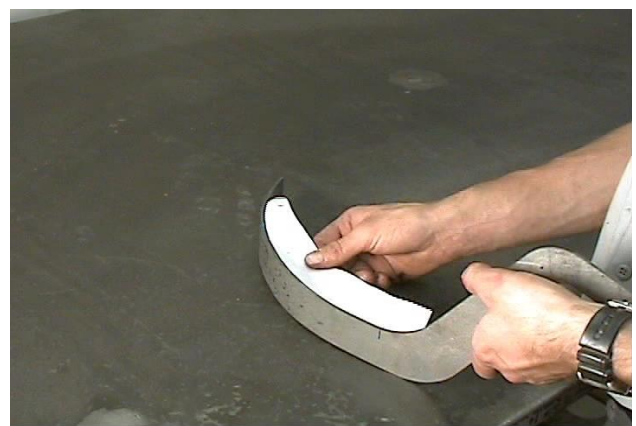
Figure 12 - Rear Template Bend Profile
