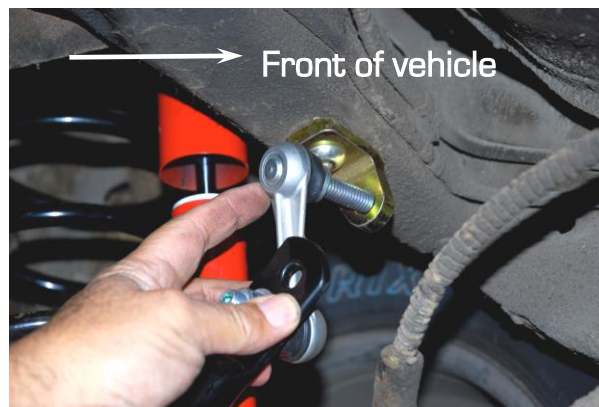
Figure 3 - Upper Link Mount ('73-'77 Applications)
