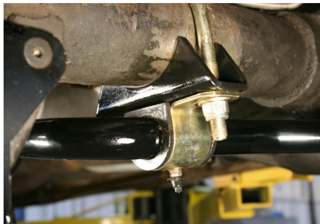
Figure 4 - Sway Bar Mounted on Rear Axle
