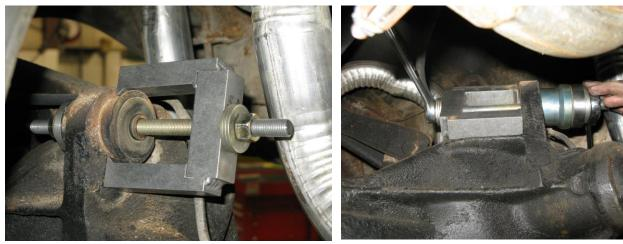
Figure 1 – Bushing removal
