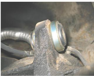
Figure 3 – Replacement Bushing Installed
