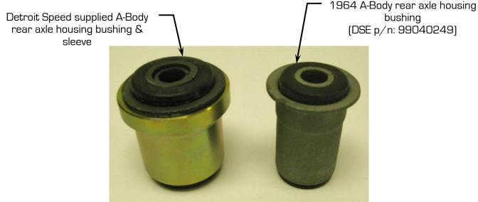
Figure 4 – Rear Axle Bushings
