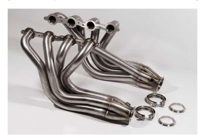
**NOTE:** When installing these headers in the DSE Hydroformed Subframe, it is required that you use the DSE LS Engine Mount Kit P/N: 060404DS.
