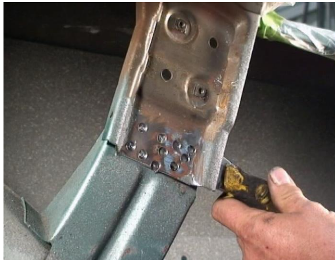
Figure 2- Separating the Passenger Side Trunk Support Flange
