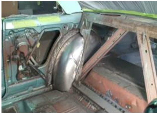
Figure 16c - Finished Modified Brace
