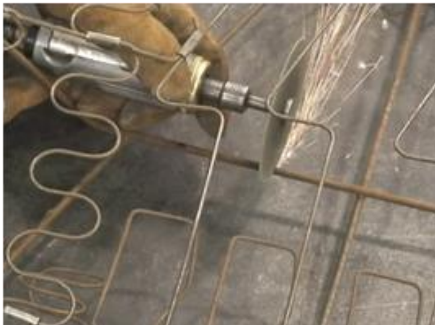
Figure 27 - Cutting the Cross Bar at the 2-1/2" Mark
