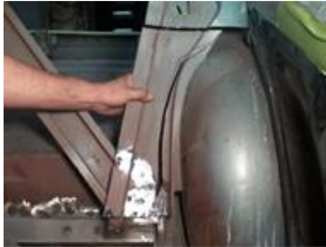
Figure 6c – Removing the Bottom Corner Flange
