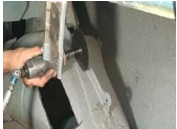
Figure 7b – Cutting the Factory Wheel Well
