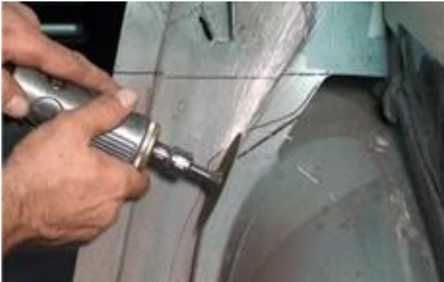
Figure 6a – Cutting the Seatback Brace
