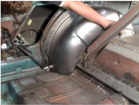
Figure 14a – Mark Surface for Weld
