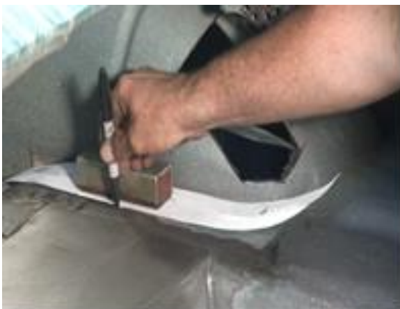
Figure 7a – Tracing the Lower Templates
