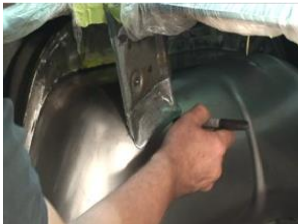
Figure 20a - Mark Driver Side for Welding
