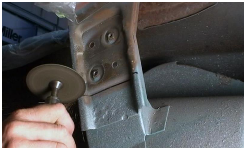
Figure 3 - Cutting the Driver Side Trunk Support Flange
