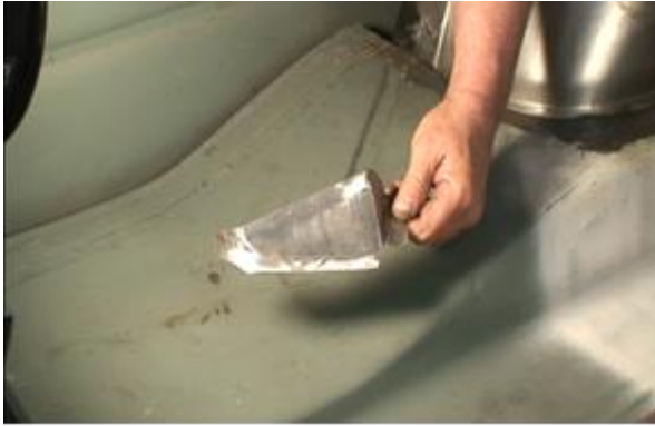
Figure 23a - Fabricate Flange for 66-67 Vehicles Figure 23b - Trimming Factory Brace & Flange
