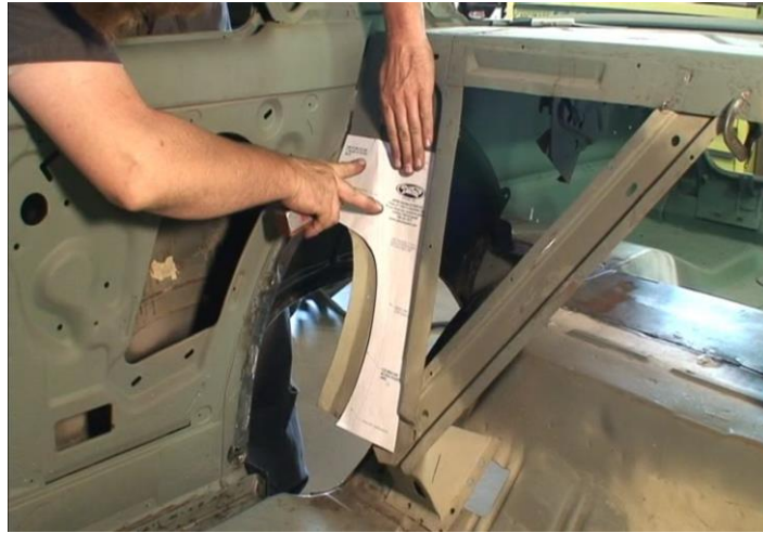
Figure 21 - Marking the Upper Seatback Brace
