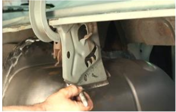
Figure 23a - Fabricate Flange for 66-67 Vehicles Figure 23b - Trimming Factory Brace & Flange
