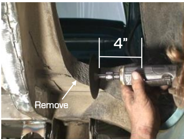
Figure 9a – Cutting the Factory Flange
