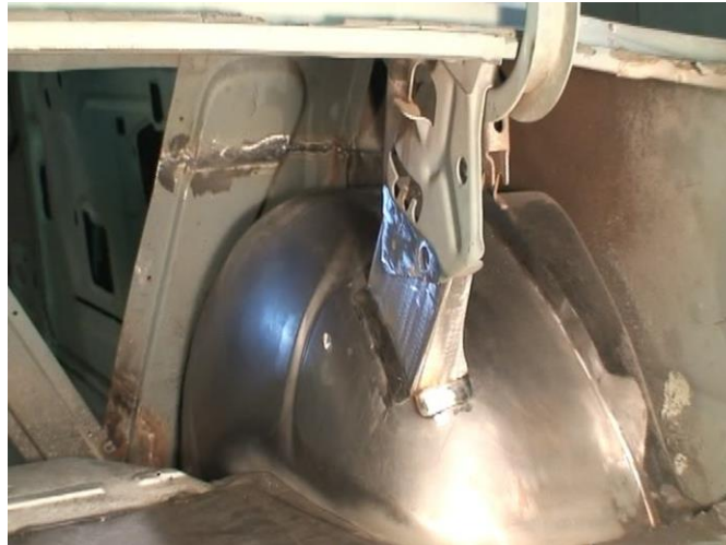
Figure 24 - Finished Passenger Side Trunk Brace
