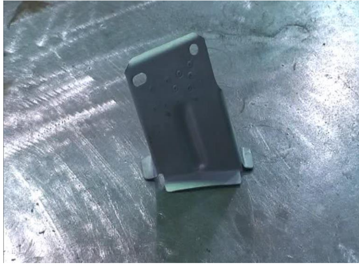
Figure 18 - Modified and Primed Factory Trunk Flange
