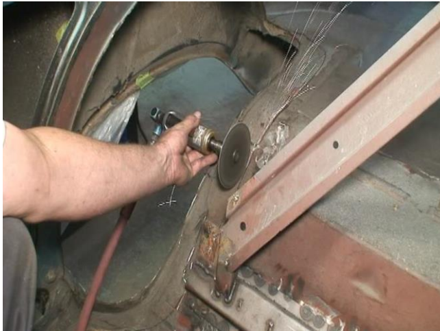
Figure 8 - Removing the Previously Traced Floor Pan Section
