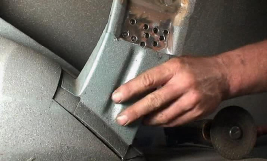
Figure 4 - Removing the Passenger Side Trunk Support Flange after Cutting
