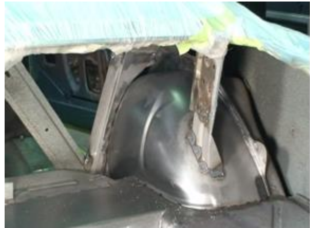
Figure 19b - Passenger Trunk Brace Flange
