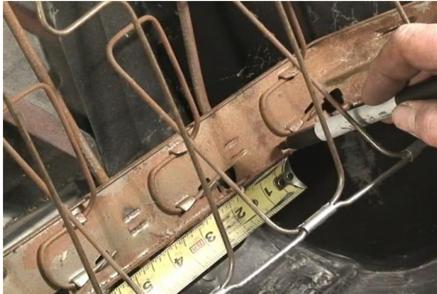
Figure 26 - Cut 2" from Top and Bottom Rail
