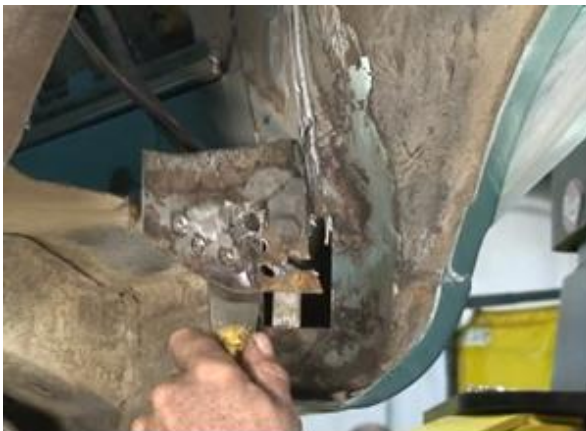
Figure 11a – Removing Forward Lap Flange
