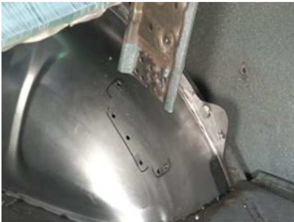
Figure 19a - Tub Marked for Flange
