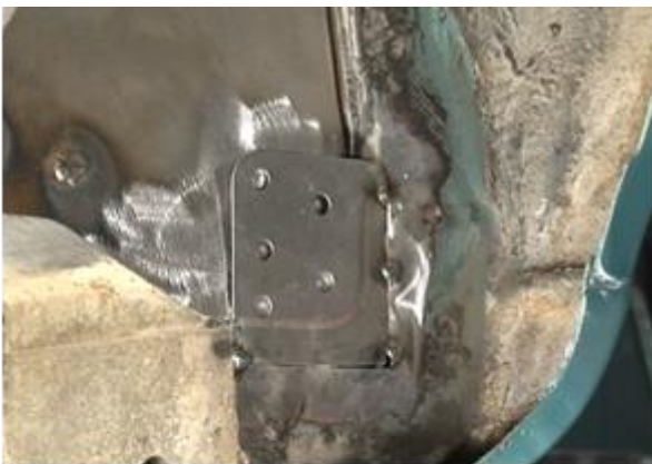
Figure 15a – Weld Front Lap Flange
