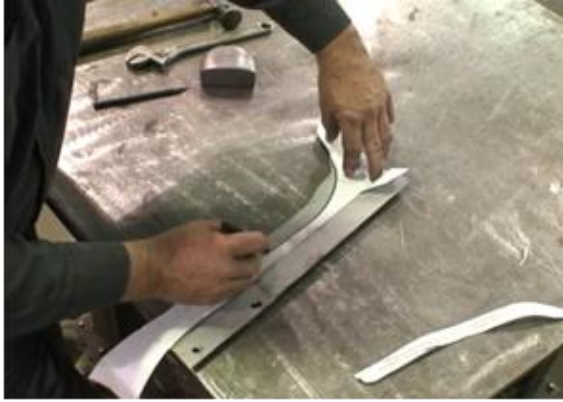
Figure 16a - Trace Template on Brace
