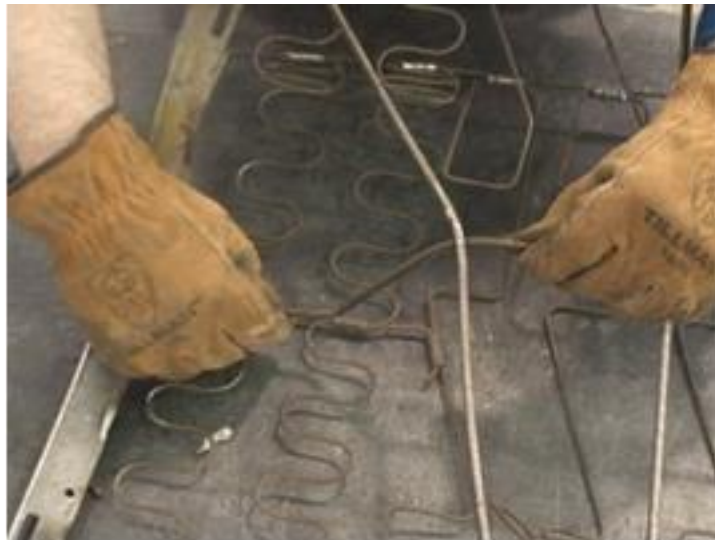
Figure 28 - Finished Flipped Cross Rod & Bent Diagonal
