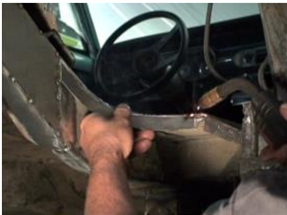
Figure 13a - Fabricate Front Flange
