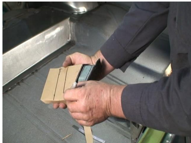
Figure 17 - Comparing Cardboard Template to Factory Trunk Flange
