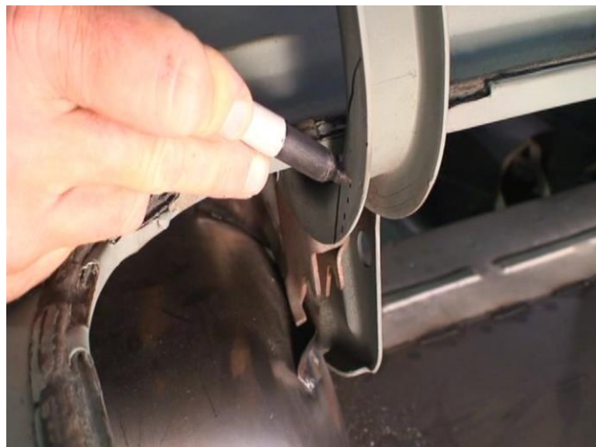
Figure 25 - Trimming Trunk Hinges for Clearance
