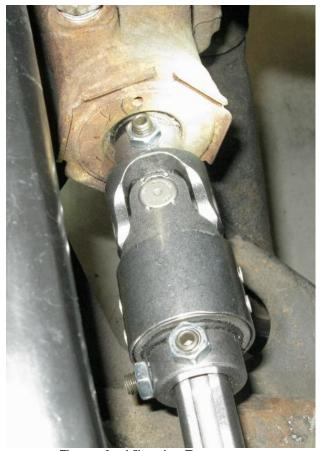
Figure 4 - Vibration Damper
