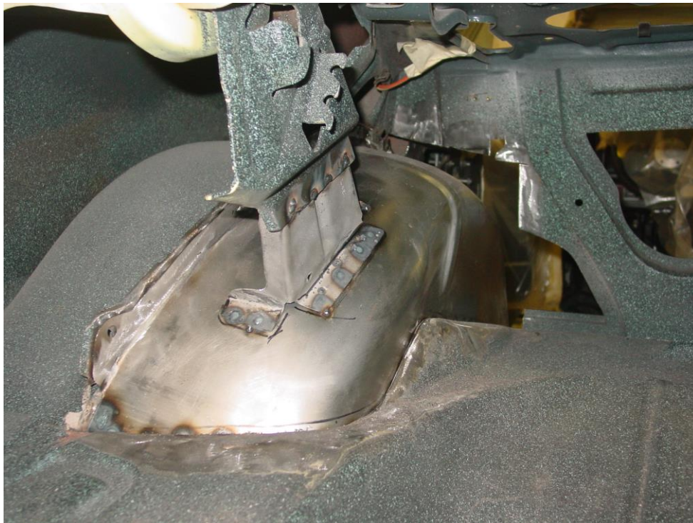
Figure 13 - Welded View (Trunk Area)
