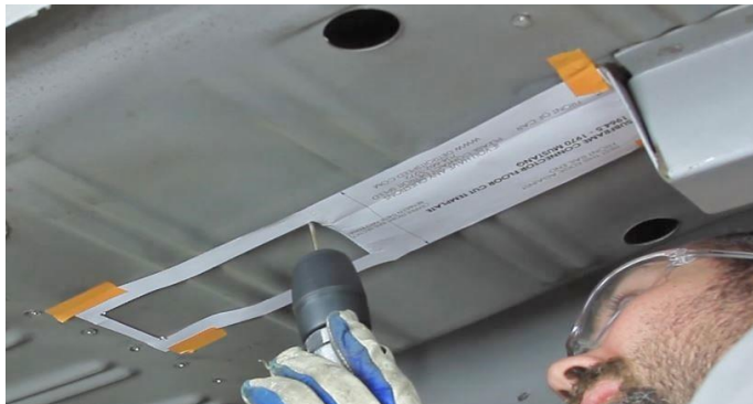
Figure 5 - Cut Floor Pan Front Frame Rail Doubler Installation
