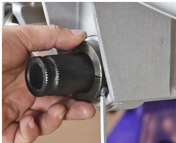
Figure 23 – Install Split Lock Collars
