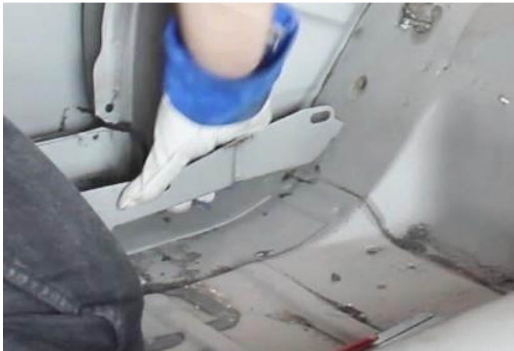
Figure 2 – Remove Interior Brackets
