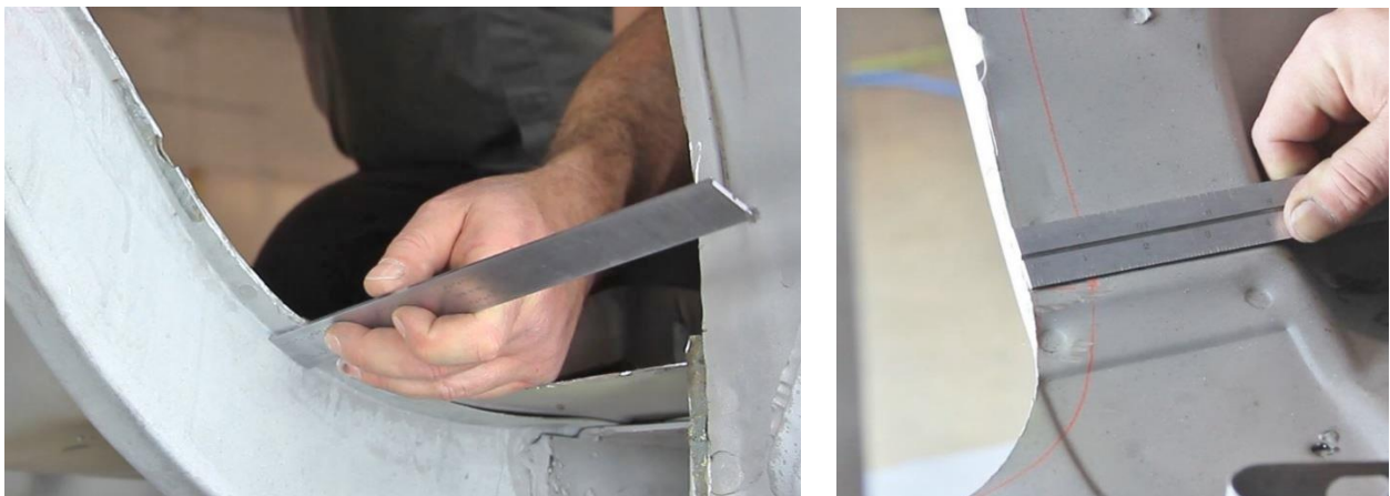
Figure 18 – Transfer Flange Dimension
