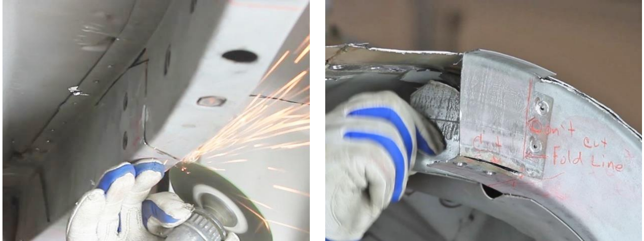
Figure 16 – Remove Frame Rail Section
