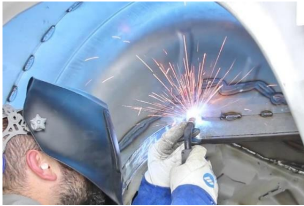
Figure 27 - Stitch Weld Mini-Tub to Frame Rail & Outer Tub Flange
