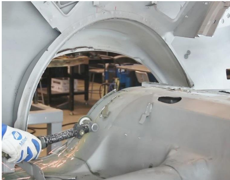
Figure 9 – Remove Floor Pan Section
