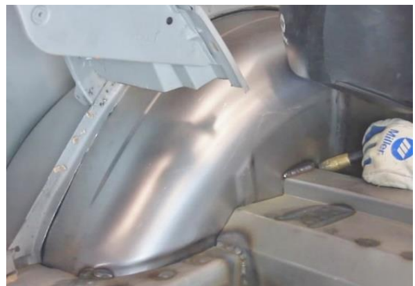
Figure 26 - Weld Mini-Tub to Stock Outer Tub
