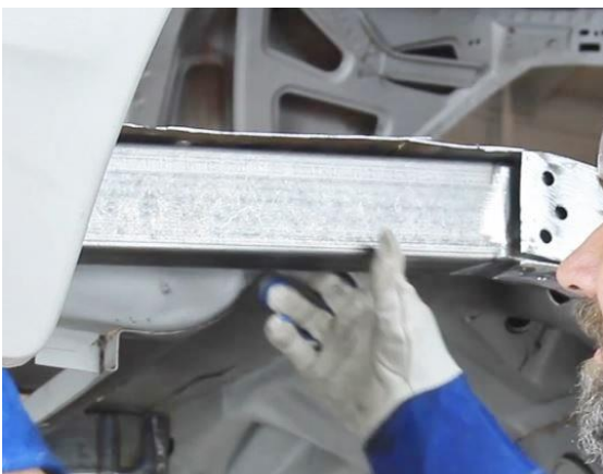
Figure 21 - Clamp Detroit Speed Frame Rail in Place
