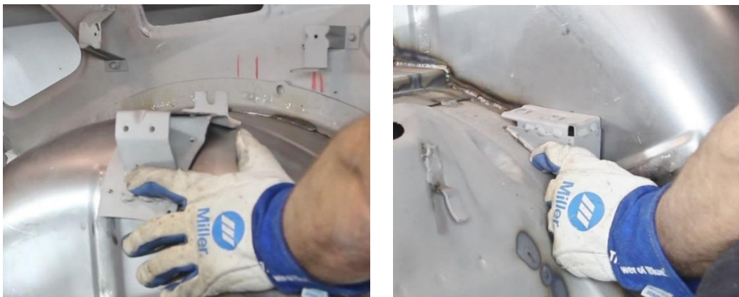
Figure 31 - Re-attach Upper & Lower Seat Brackets
