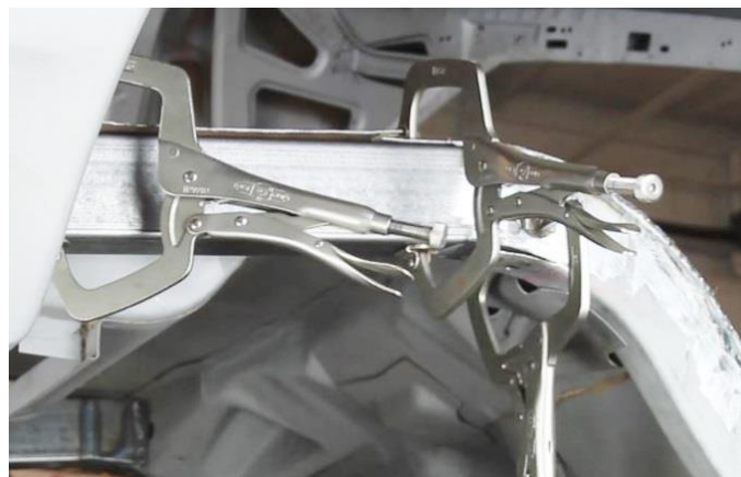
Figure 21 - Clamp Detroit Speed Frame Rail in Place
