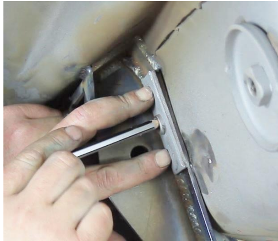
Figure 33 – Re-position the Seat Belt Anchor
