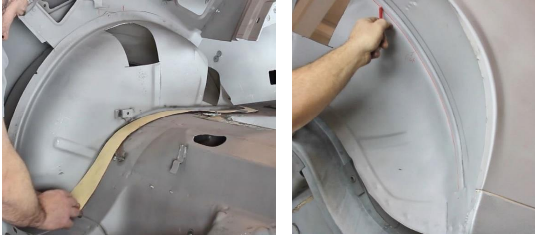
Figure 5 - Trace Floor Pan Cut Template
