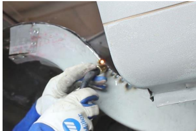
Figure 20 - Cut & Weld Sheet Metal Layers
