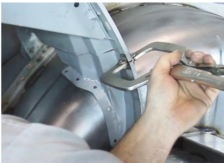
Figure 29 - Weld Rear Seat Support to Mini-Tub (Fastback)
