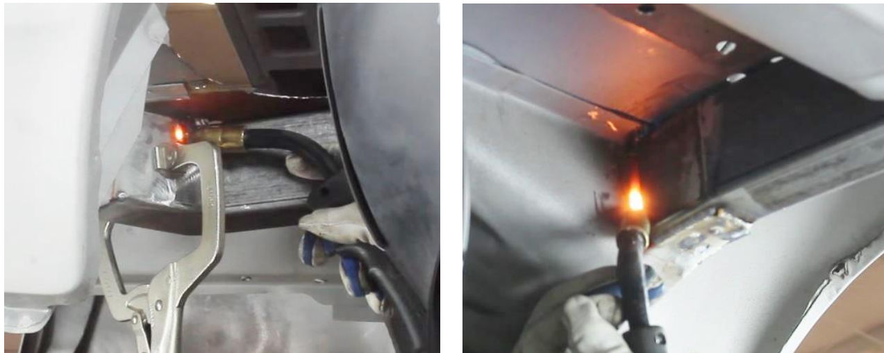
Figure 22 - Weld-In Detroit Speed Frame Rail Section
