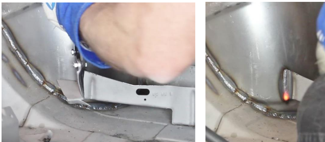
Figure 32 - Re-attach Rear Interior Panel Bracket
