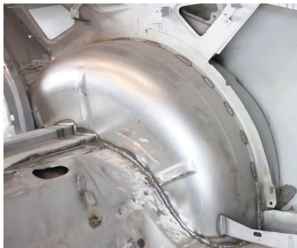
Figure 34 – Installed Detroit Speed Mini-Tub
