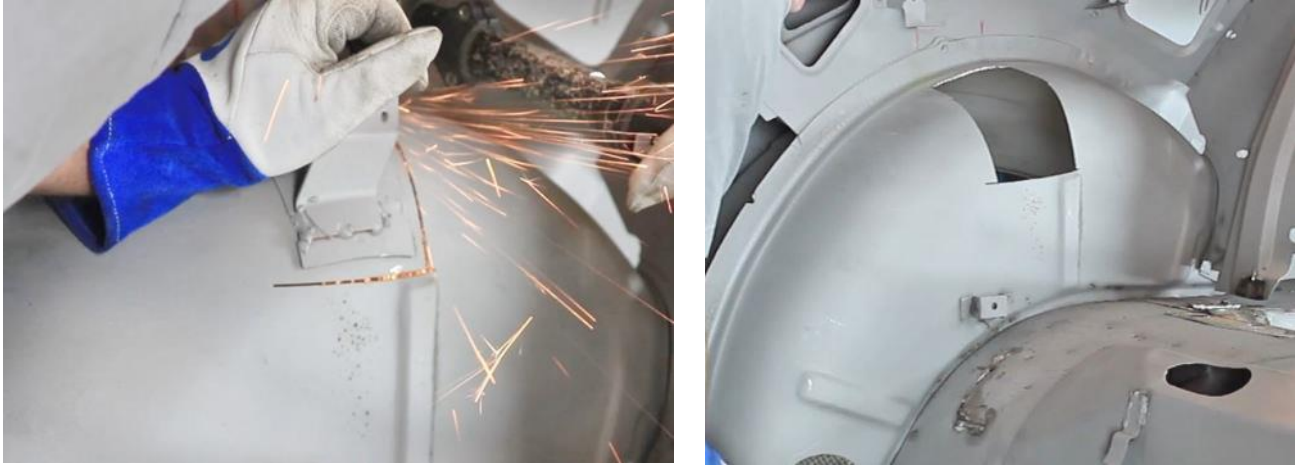
Figure 1 – Remove Lower & Upper Seat Brackets
