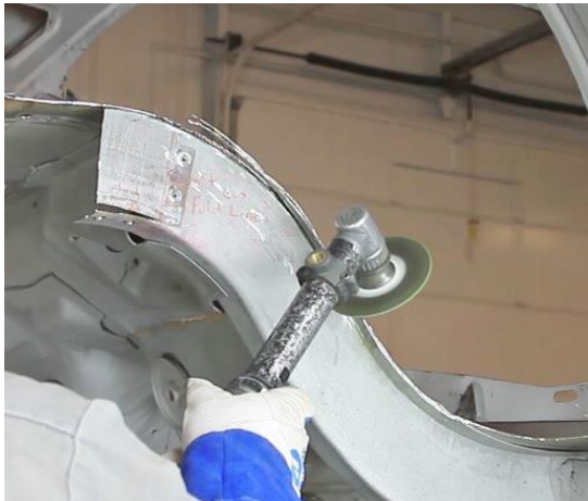
Figure 20 - Cut & Weld Sheet Metal Layers
