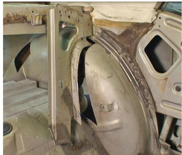
Figure 4 - Remove Seat Support & Decklid Hinge (Coupe)
