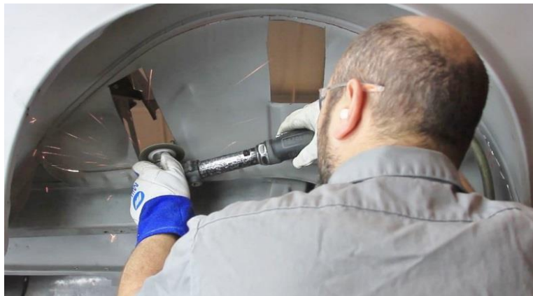
Figure 6 - Cut Out & Remove Inner Tub
