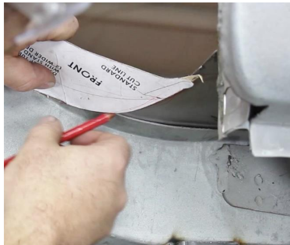
Figure 17 – Connect Frame Rail to Inner Tub Cut-Out
