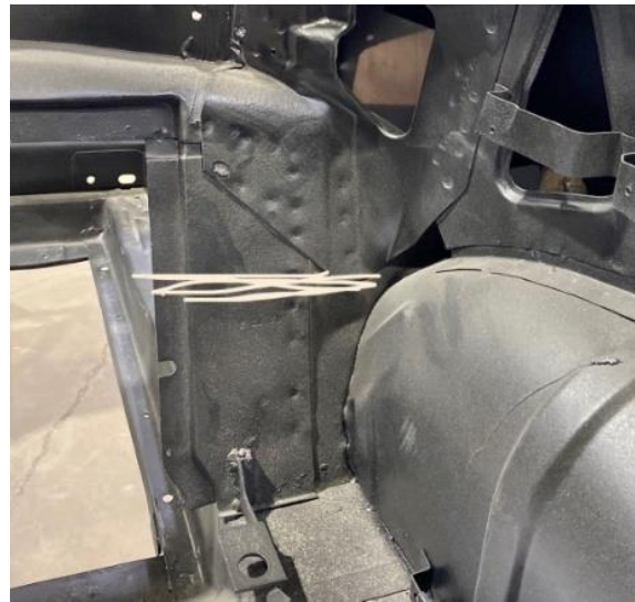
Figure 3b - Remove Seat Support (1965 Fastback)
