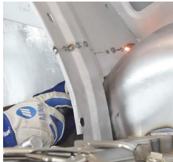
Figure 29 - Weld Rear Seat Support to Mini-Tub (Fastback)
