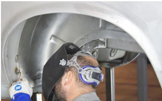
Figure 26 - Weld Mini-Tub to Stock Outer Tub
