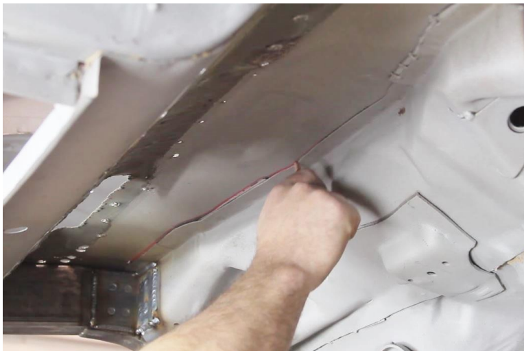
Figure 1 – Mark Floor Pan Cut Line (Underneath Vehicle)
