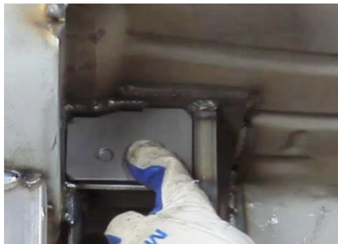
Figure 18 – Locate Lower Link Closeout
