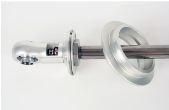
Figure 39 - Removing the Upper Spring Seat
