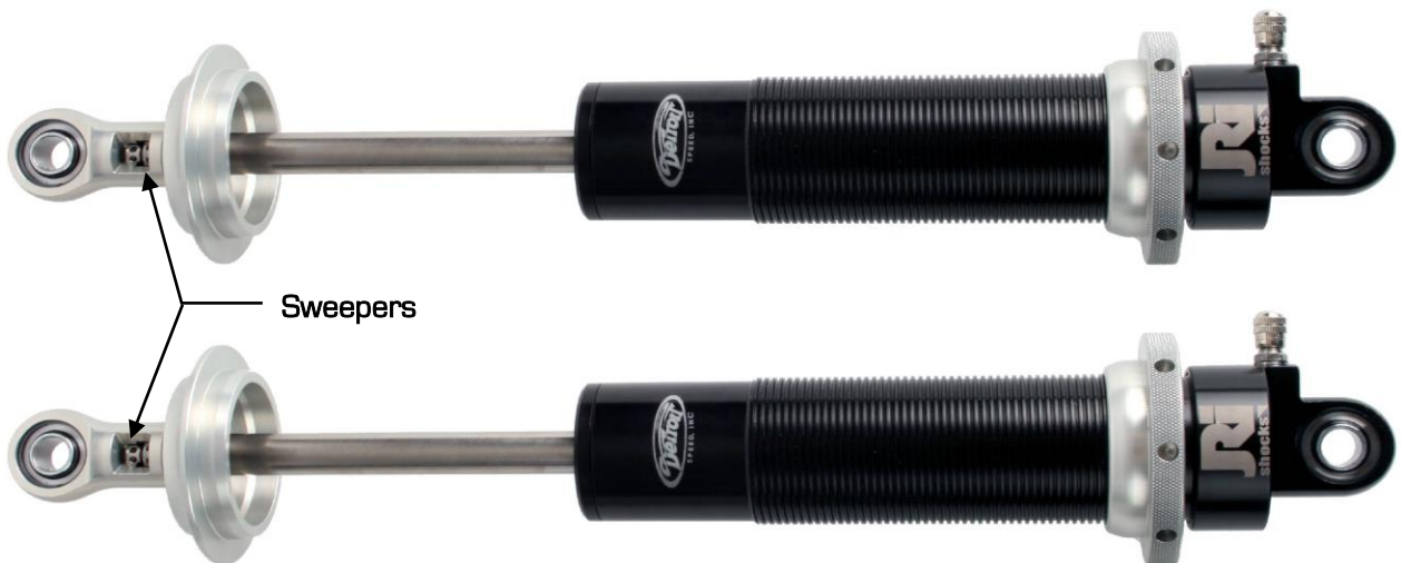
Figure 52a - Detroit Speed Double Adjustable Shock
