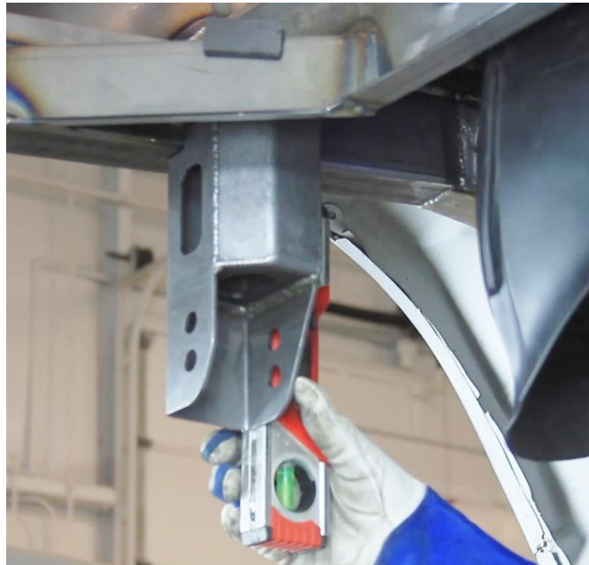
Figure 28 – Weld Track Bar Body Bracket
