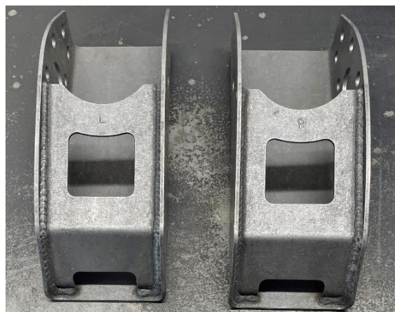
Figure 11 - Front Upper Link Mounting Bracket
