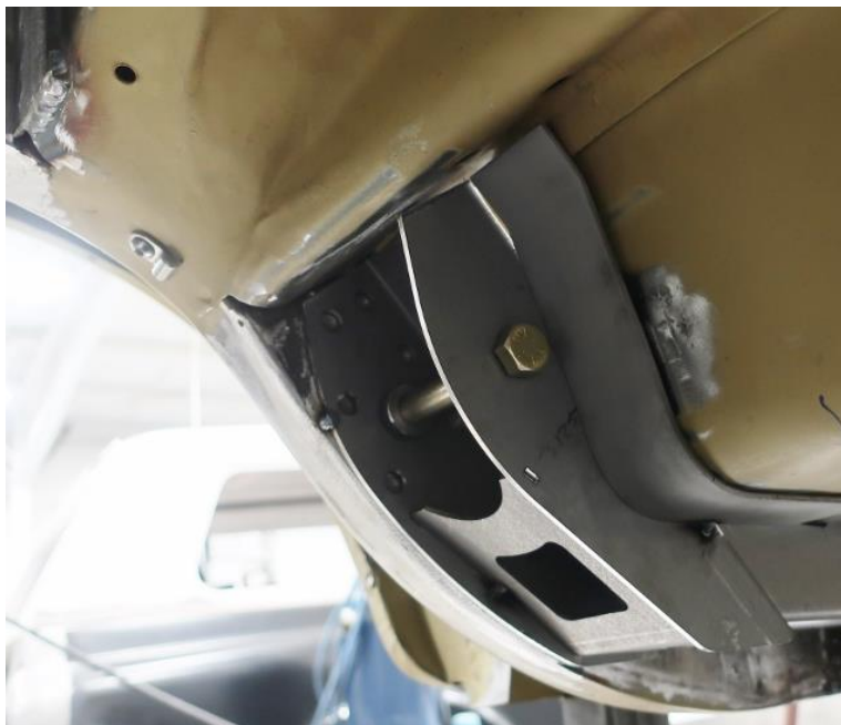
Figure 13 - Tack Weld Upper Link Pocket
