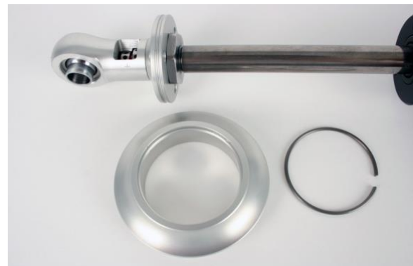
Figure 40 - Upper Spring Seat & Retaining Ring
