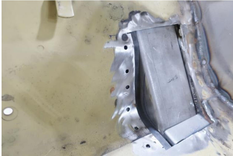
Figure 12 - Pocket Floor for Clearance
