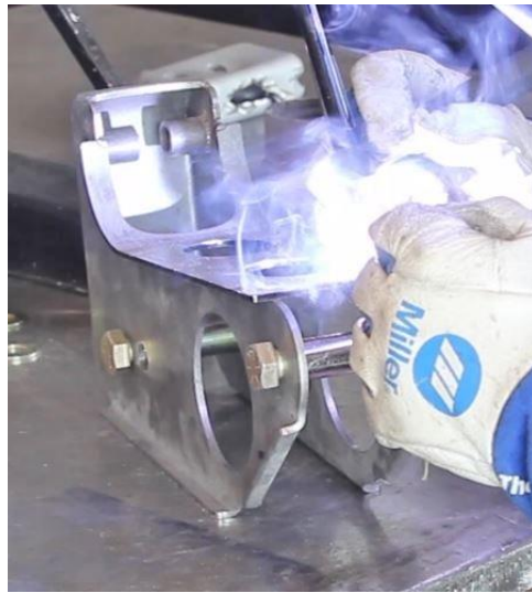
Figure 30 - Weld Axle Bracket Reinforcement
