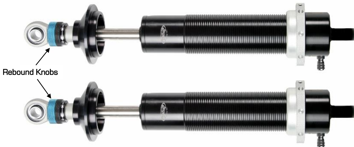
Figure 51a- Detroit Speed Single Adjustable Shock
