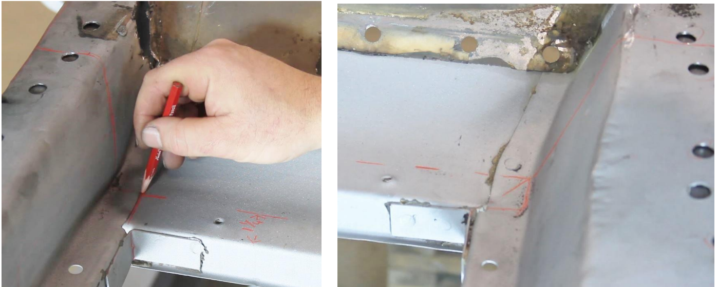
Figure 2 - Mark Floor Pan Cut Lines (Trunk)
