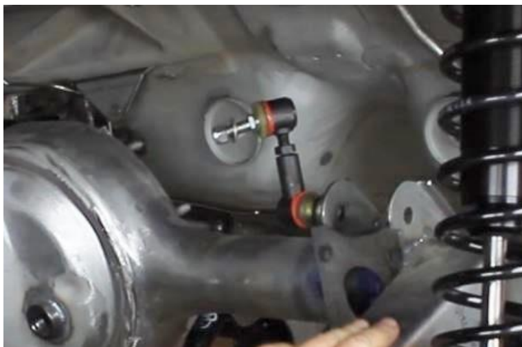
Figure 43 - Install Sway Bar End-Links onto Axle Brackets
