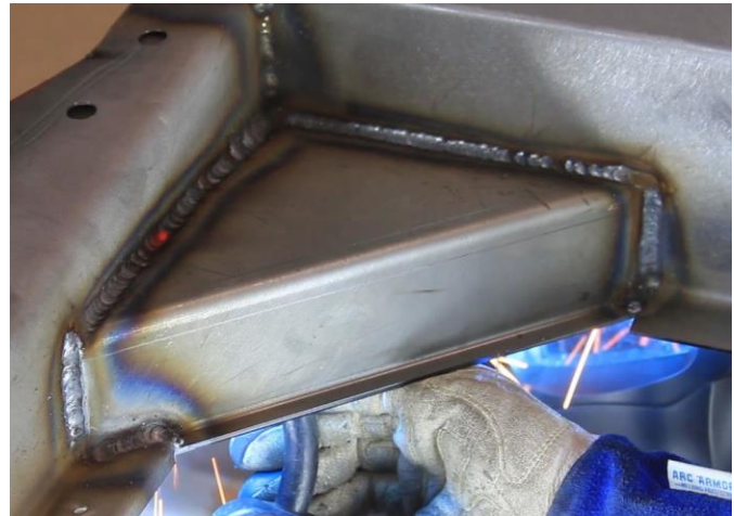
Figure 26 - Trim & Weld Front Trunk Closeouts
