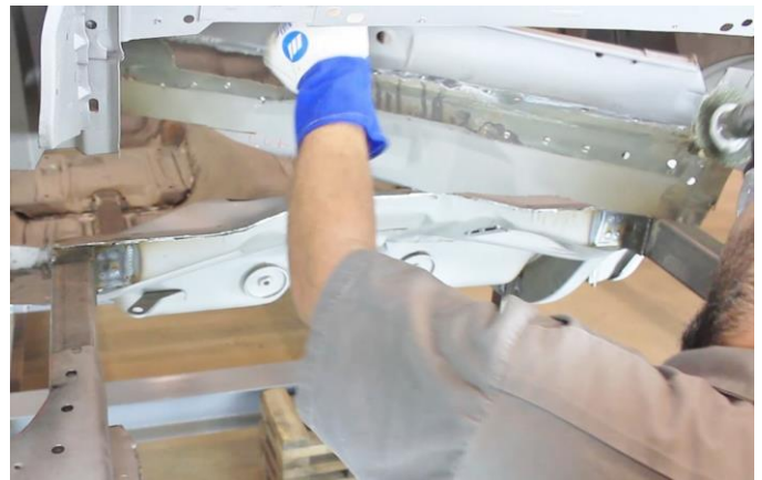
Figure 5 – Remove Trunk Floor Section
