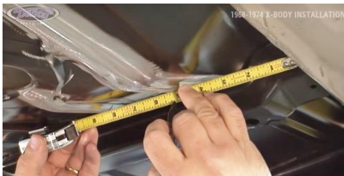
Figure 5 - Measure 5\text{-}1/8" Inboard of Pinch Weld
