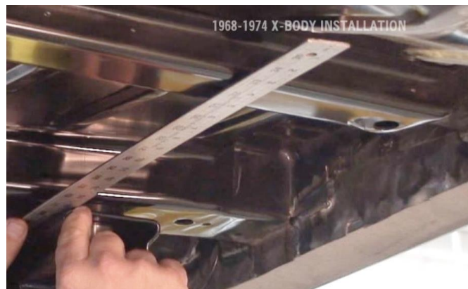
Figure 4 - Measure 15\text{-}1/8" From Subframe
