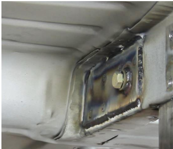
Figure 5 - Weld Outboard Torque Box Plate
