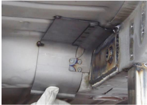
Figure 8 - Weld Top Assembly
