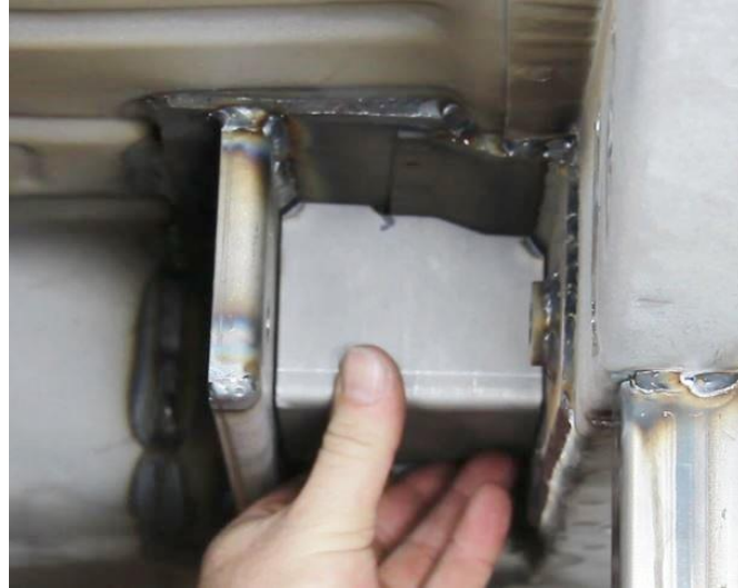
Figure 11 - Fit Bottom Torque Box Plate
