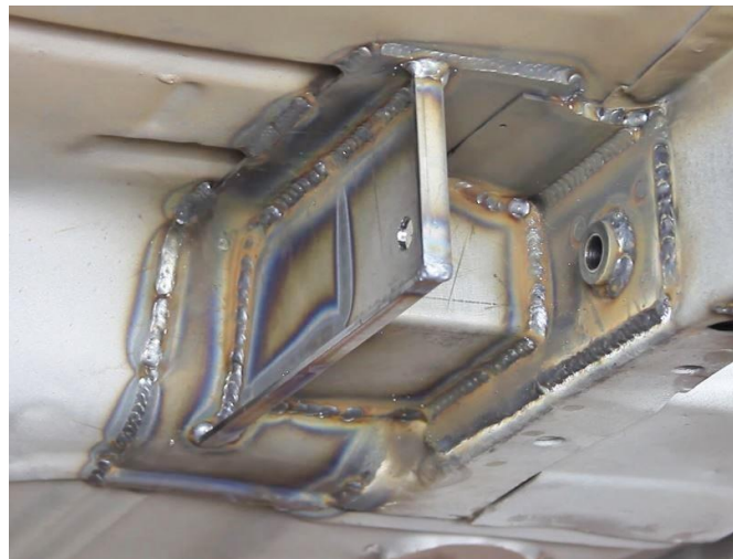
Figure 12 - Finish Weld Torque Box
