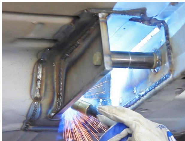
Figure 10 - Weld Inboard Plate
