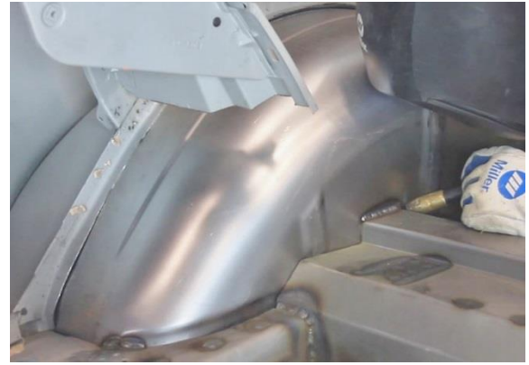
Figure 26 – Weld Mini-Tub to Stock Outer Tub
