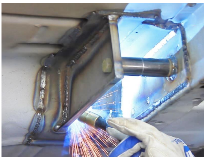
Figure 43 - Weld Inboard Plate
