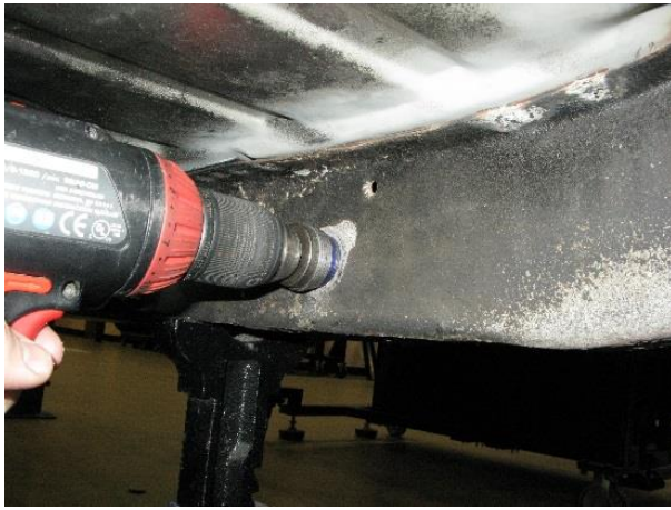
Figure 36 - Remove Factory Crush Tube
