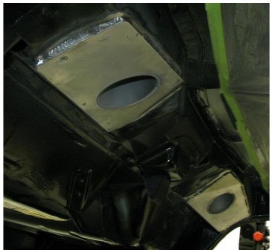
Figure 52 - Weld Upper Shock Mounts
