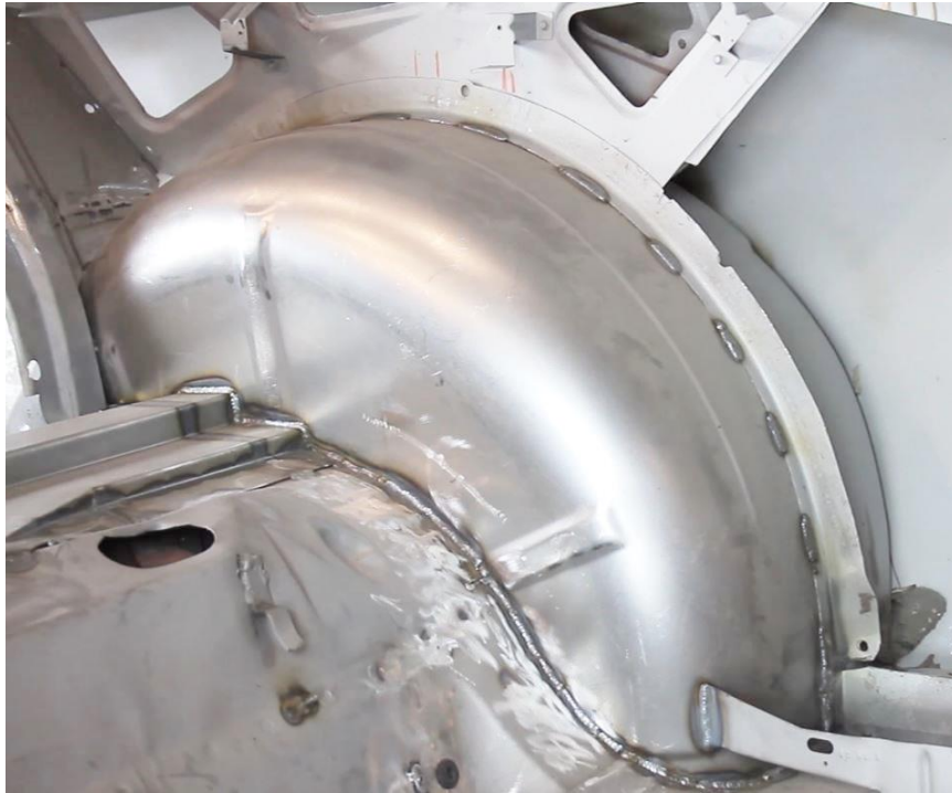
Figure 34 - Installed DSE Mini-Tub
