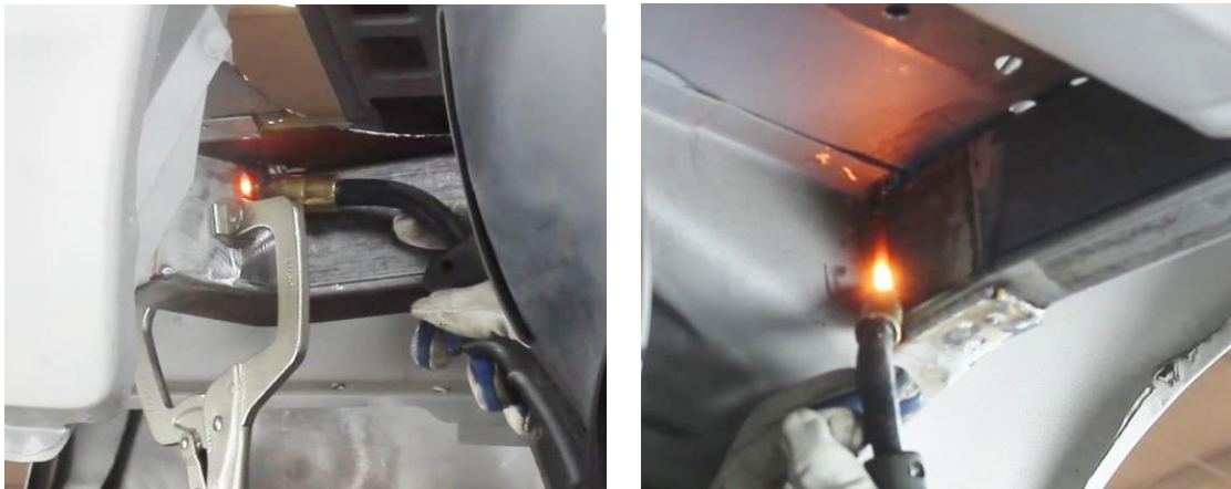
Figure 22 – Weld-In DSE Frame Rail Section
