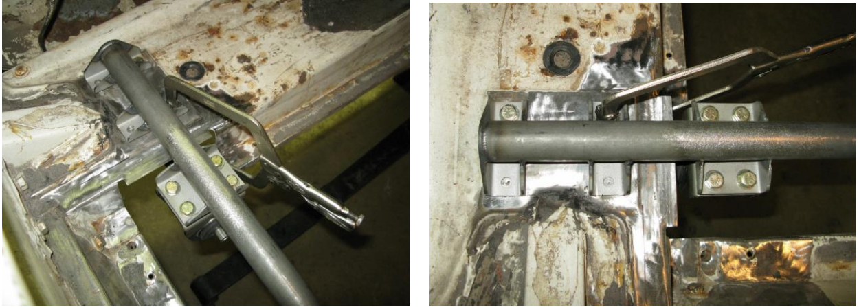
Figure 49 - Drill Support Tube Mount
