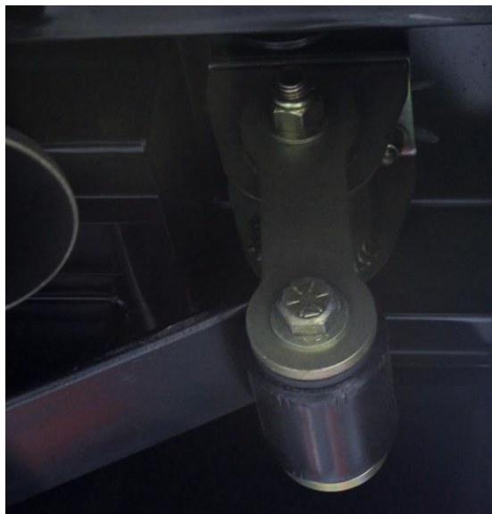
Figure 57 - Install Leaf Springs
