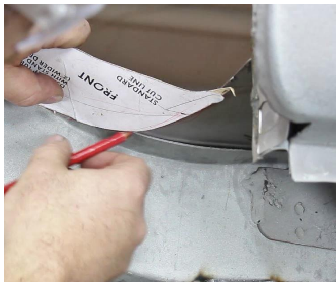
Figure 17 - Connect Frame Rail to Inner Tub Cut-Out
