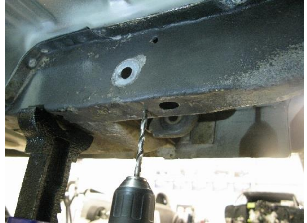
Figure 36 - Remove Factory Crush Tube
