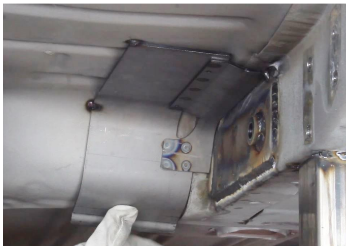
Figure 41 - Weld Top Assembly
