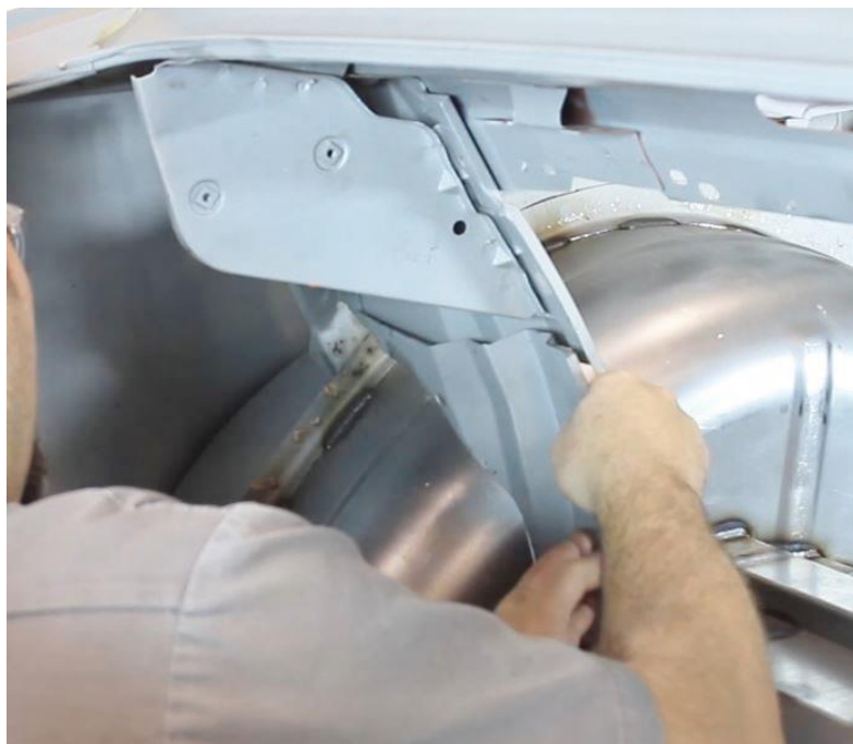
Figure 28 – Modify Rear Seat Support
