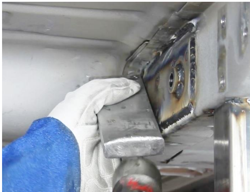
Figure 40 – Modify Floor Pan
