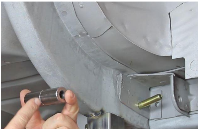
Figure 38 - Install Weld Spacer
