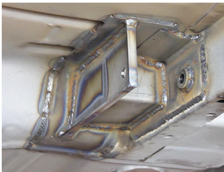
Figure 45 – Finish Weld Torque Box
