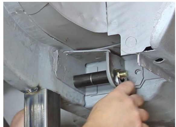
Figure 38 - Install Weld Spacer
