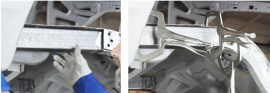
Figure 21 – Clamp DSE Frame Rail in Place
