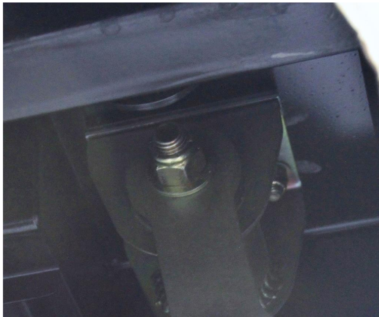
Figure 53 – Install Shackle Mounts
