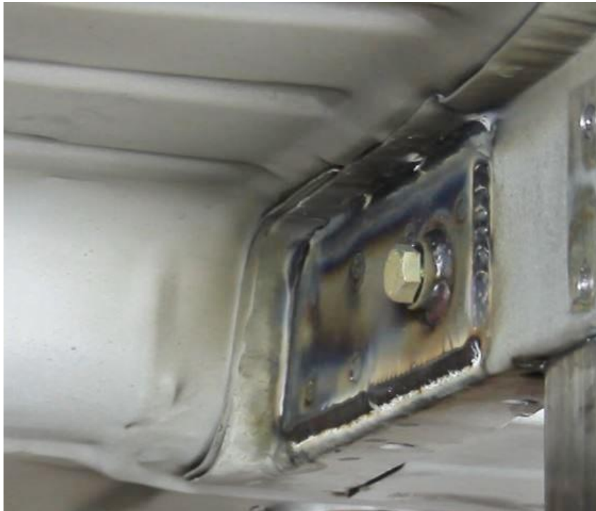
Figure 39 – Weld Outboard Torque Box Plate
