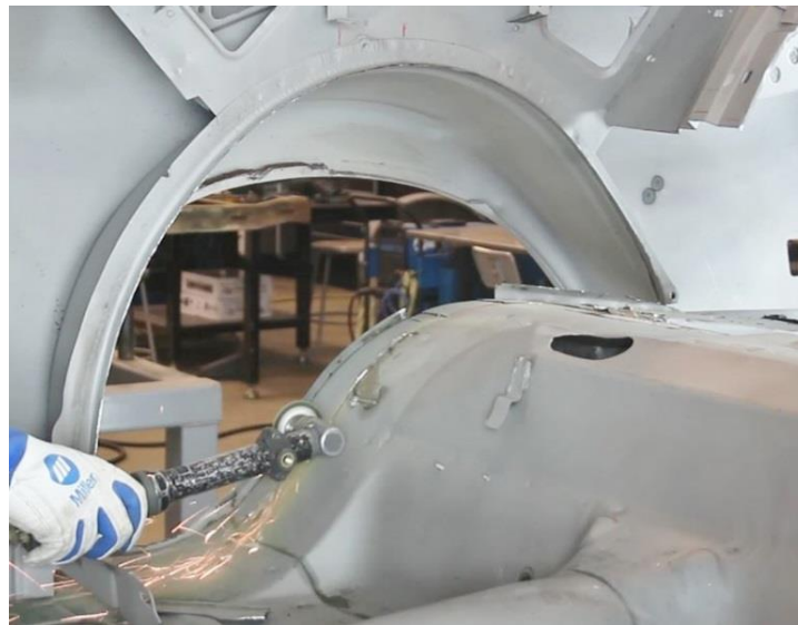
Figure 9 - Remove Floor Pan Section
