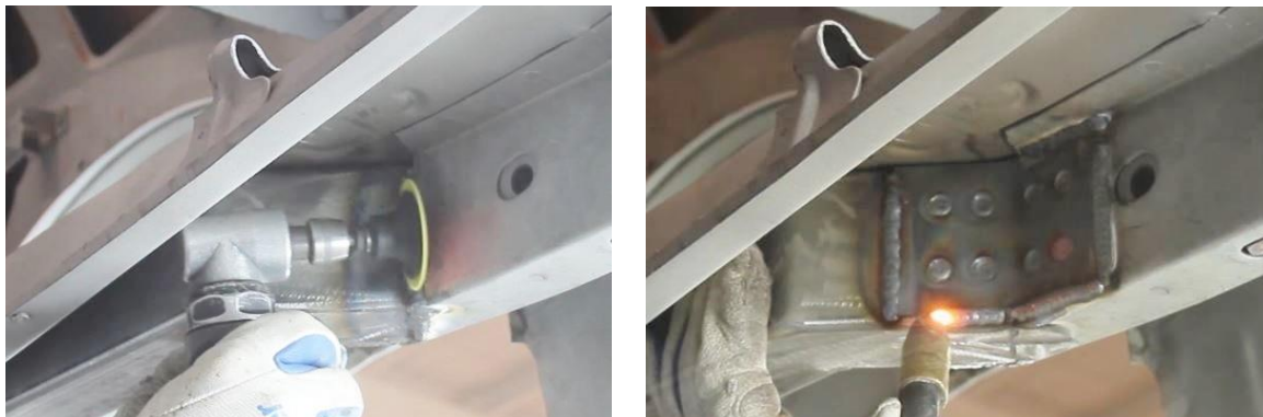
Figure 23 – Weld Inside Frame Rail Doubler Plate
