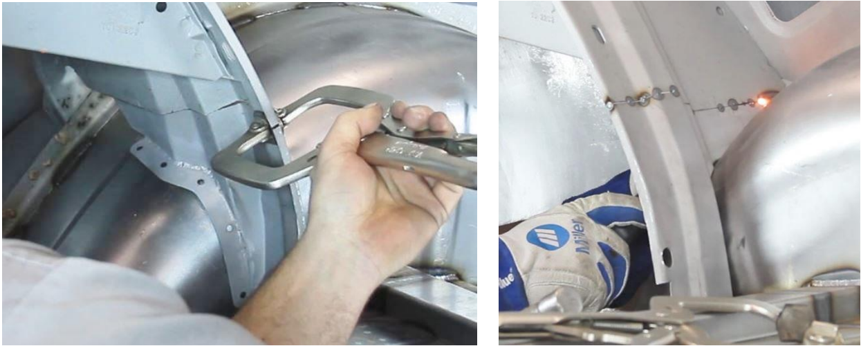
Figure 29 – Weld Rear Seat Support to Mini-Tub (Fastback)
