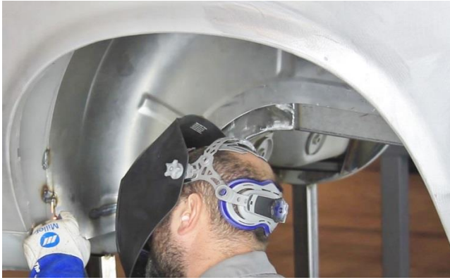
Figure 26 – Weld Mini-Tub to Stock Outer Tub
