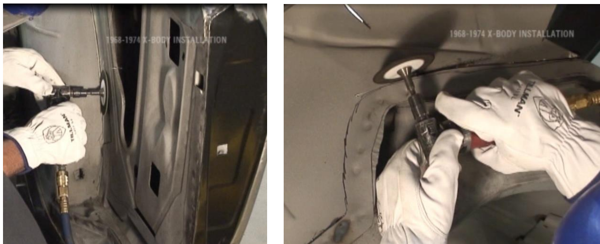
Figure 13 – Cut Pre-Marked Lines
