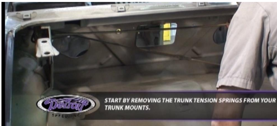
Figure 1 – Removing the Torsion Springs
