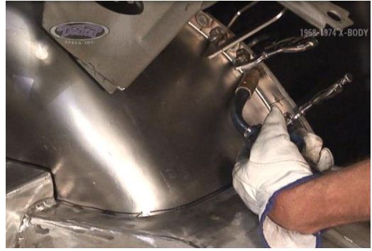
Figure 38 – Clamp and Weld to the Vehicle
