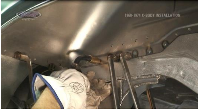
Figure 38 – Clamp and Weld to the Vehicle
