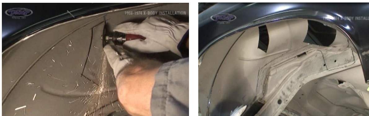
Figure 15 – Remove the Seat Brace
