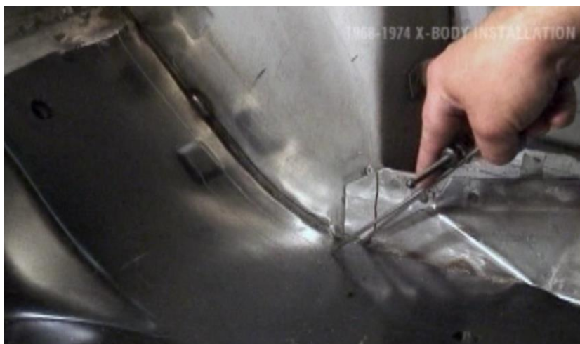
Figure 4 – Mark the Flange Bend Line
