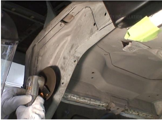
Figure 17 - Cutting along the Framerail
