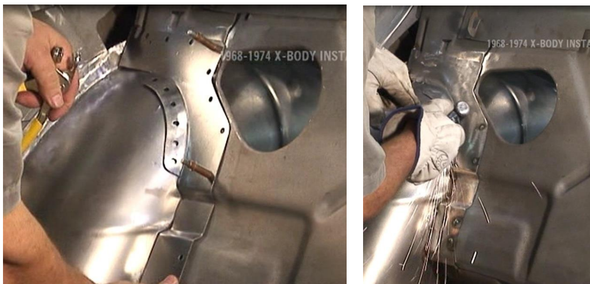
Figure 42 – Weld and Grind Seat Back Brace
