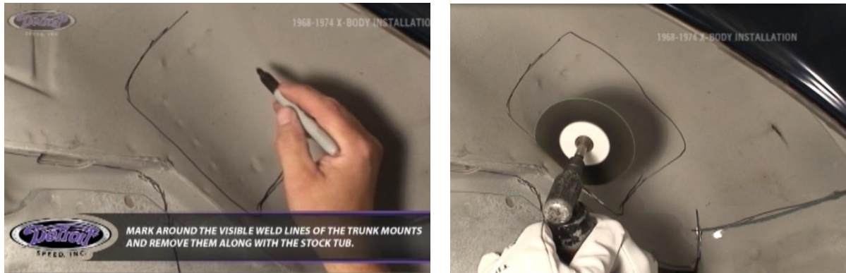
Figure 11 – Mark the Trunk Mounts
