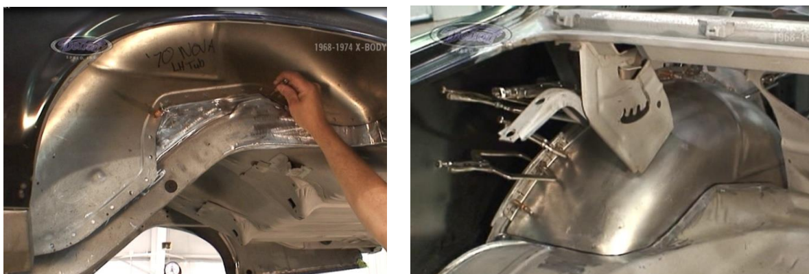
Figure 28 - Secure the Mini-Tub for Welding
