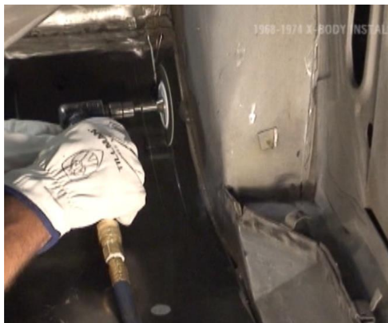
Figure 14 – Cut 1-1/4" Marked Lines
