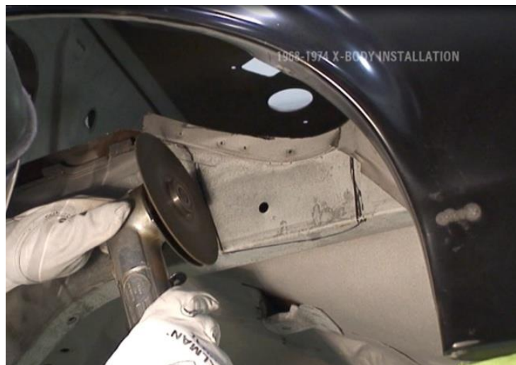
Figure 18 - Notch the Framerail
