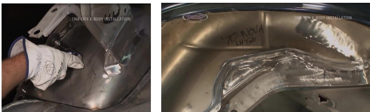
Figure 33 – Finish Grind Mini-Tub
