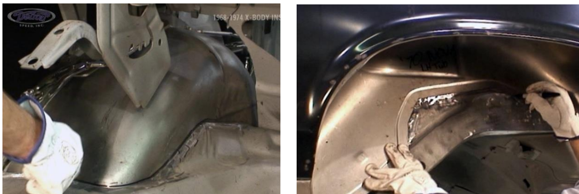
Figure 26 - Mark the Mini-Tub
