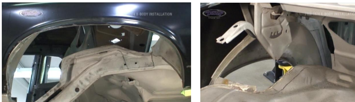
Figure 16 – Stock Inner Tub Removed
