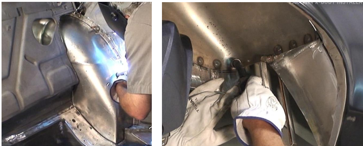
Figure 29 – Welding the Mini-Tub
