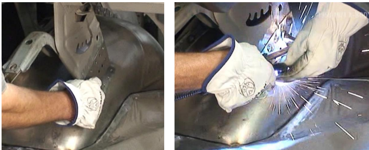
Figure 32 – Fabricate and Weld the Decklid Support
