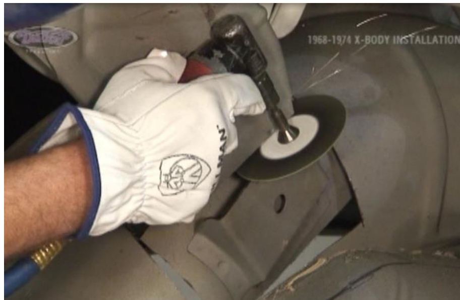
Figure 12 – Cut and Remove the Hinge Mount
