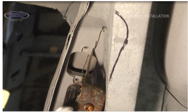
Figure 17 - Cutting along the Framerail
