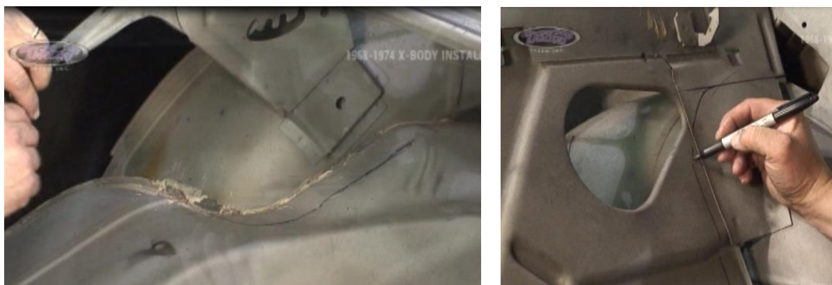
Figure 3 – Mark the Cut Lines
