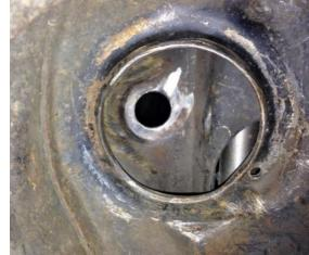
Figure 6 - Remove Sharp Edges/Burrs
