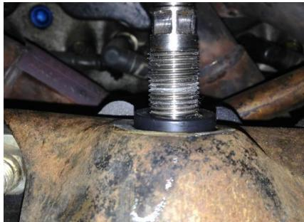
Figure 7 - Lower Shock Bushing
