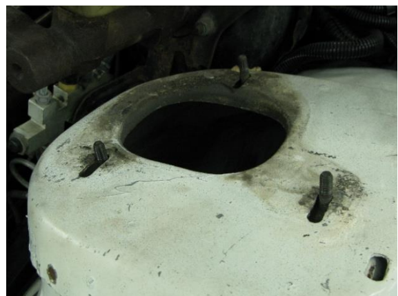
Figure 2 - Remove the Upper Strut Mount Assembly
