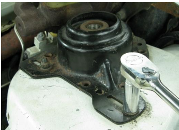
Figure 2 - Remove the Upper Strut Mount Assembly
