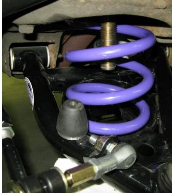
Figure 4 - Weight Jack Assembly Installed
