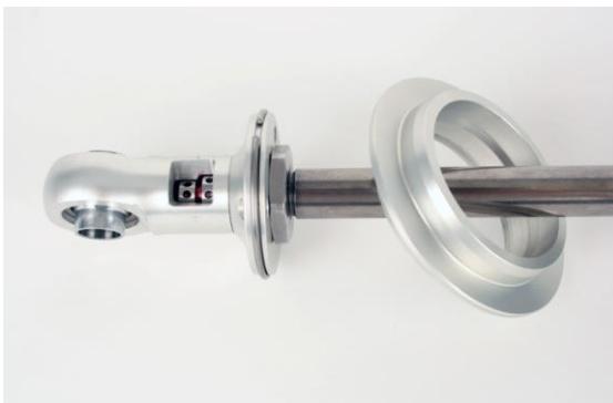
Figure 7 – Remove Upper Spring Seat
