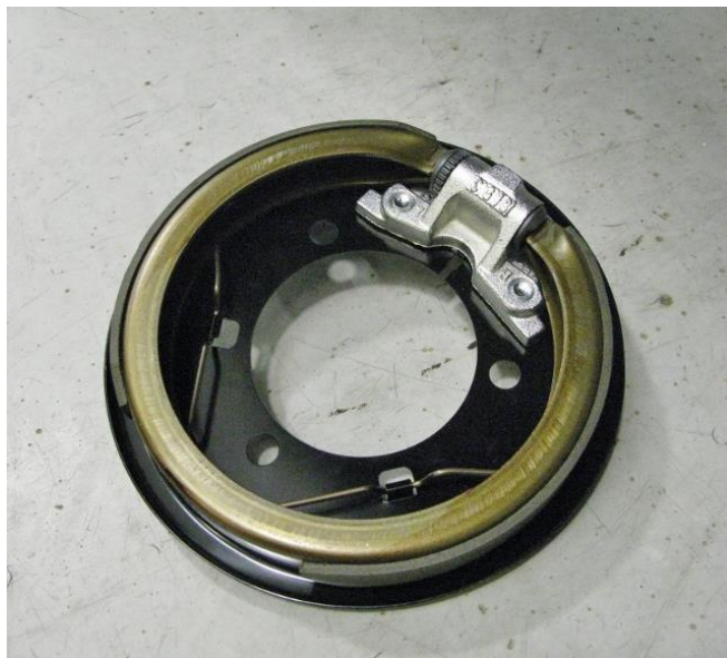
Figure 6 – Remove Park Brake Piston Bolts
