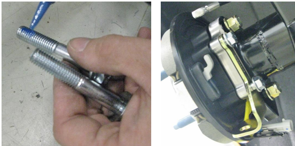
Figure 8 – Install Park Brake Cable Bracket (Driver Side)
