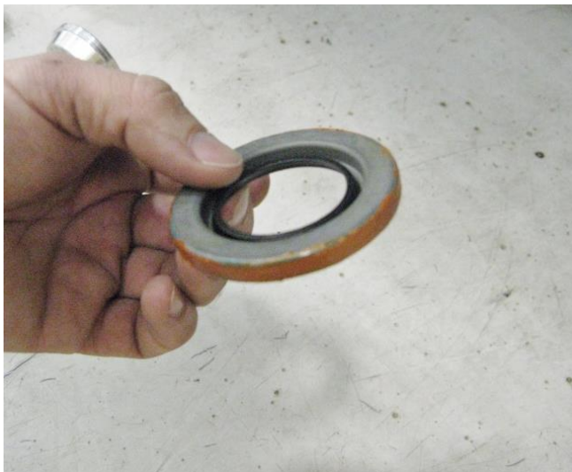
Figure 3 - Use RTV on the Axle Seals
