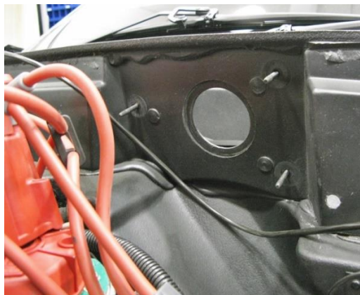
Figure 2 – Remove Original Wiper Motor
