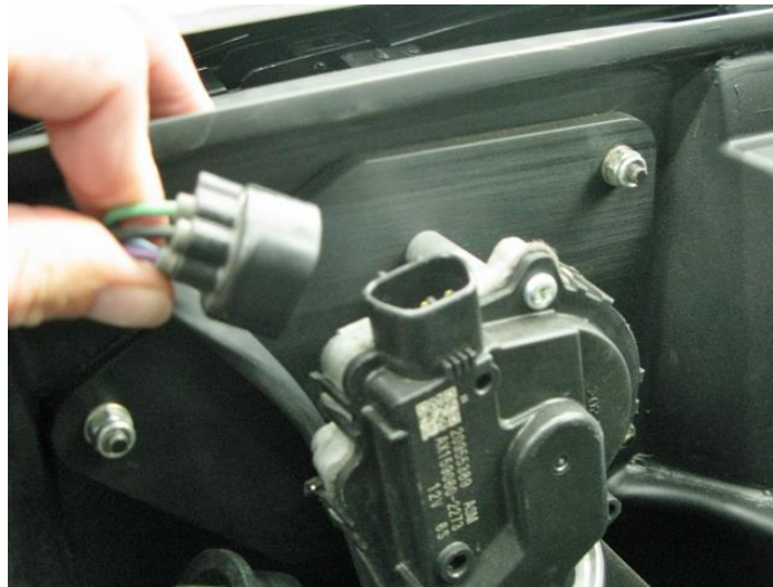
Figure 18 - Install Wiper Motor Connector
