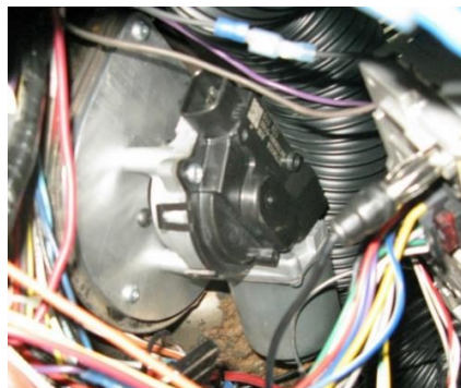
Figure 5 - Attach Wiper Motor to Firewall
