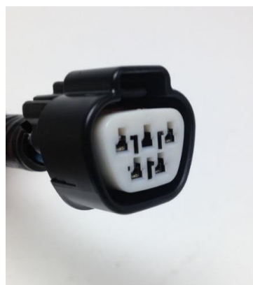
Figure 10 – Install Wiper Motor Connector
