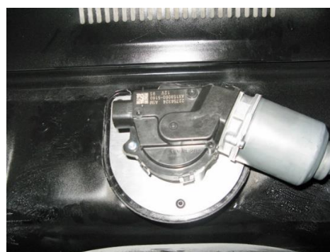
Figure 5 - Attach Wiper Motor to Firewall
