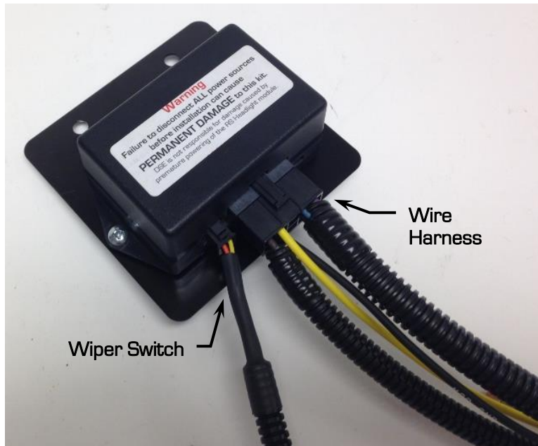
Figure 13 – Connect Wiper Switch & Harness to Module
