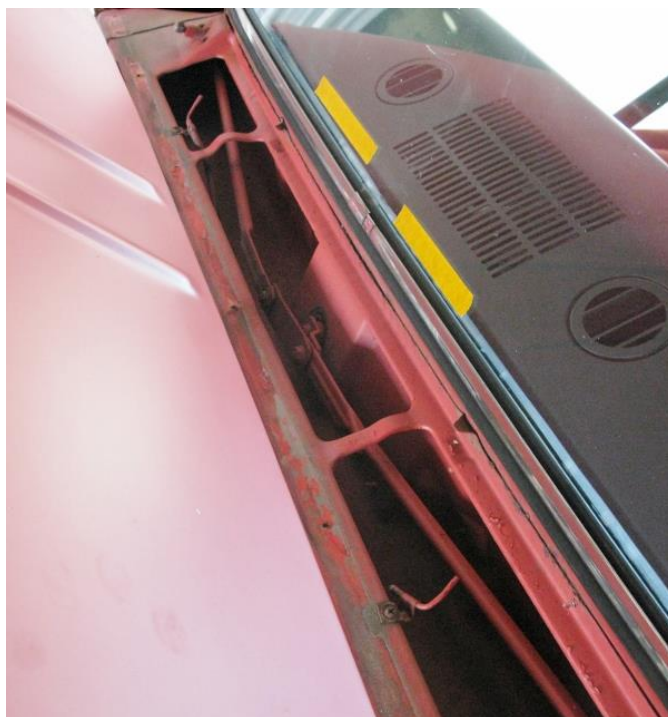
Figure 1 - Remove Cowl Panel
