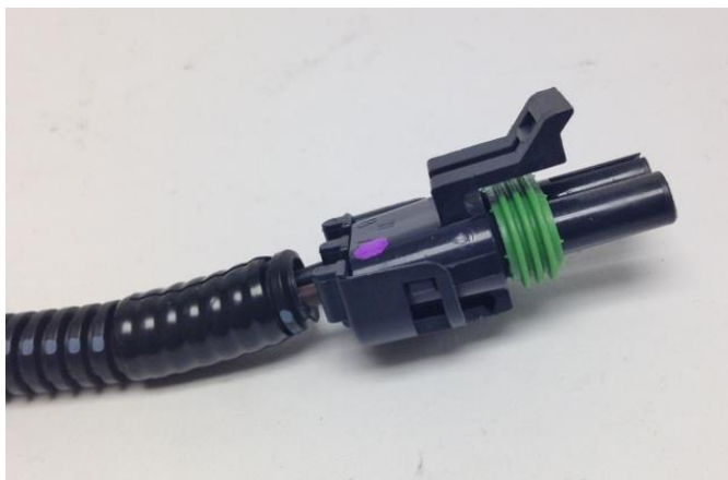
Figure 11 - Washer Pump Connection
