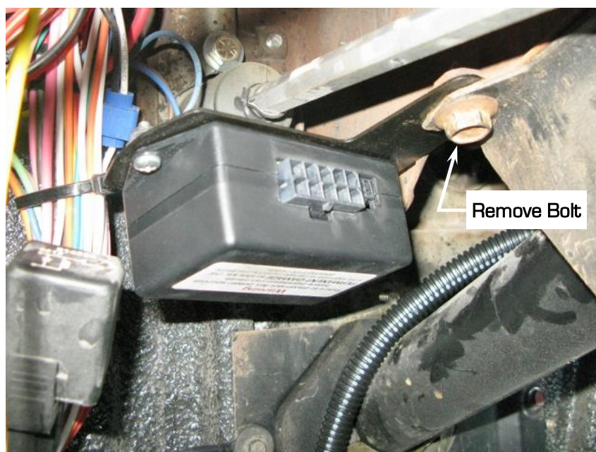
Figure 12 - Install Module & Mounting Plate
