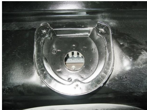
Figure 4 - Remove Factory Wiper Motor
