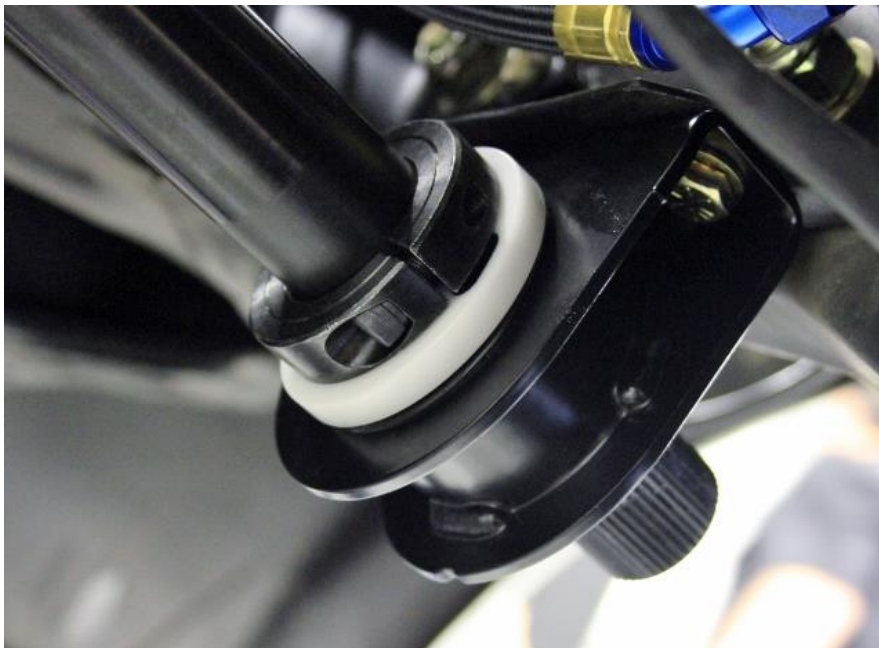
Figure 29 – Install Sway Bar Split Lock Collars
