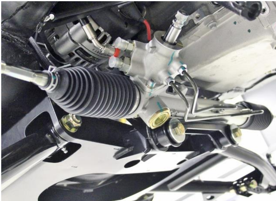
Figure 23 - Install Rack & Pinion
