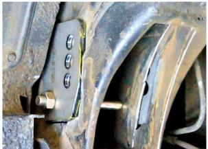
Figure 11 – Verify Frame Rail Modification
