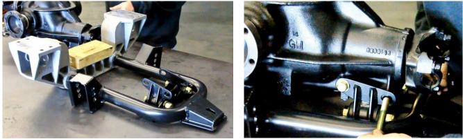
Figure 79 – IRS Lower Cradle/Rear Differential Assembly
