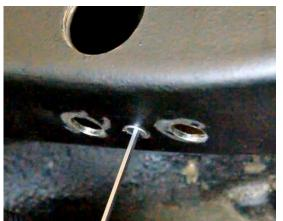
Figure 58 - Drill & Chamfer Nut Plate Locators
