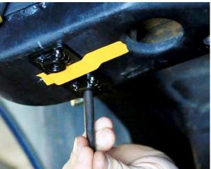
Figure 62 - Transfer Punch Nut Plate Location
