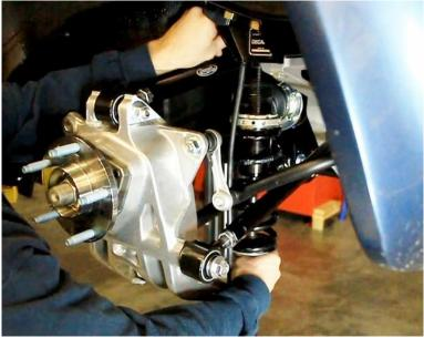
Figure 111 - Install Upper Shock Bolt & Spacer
