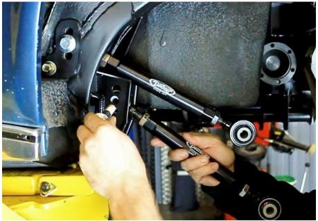
Figure 95 – Install the IRS Lower Trailing Links
