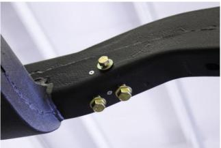
Figure 49 – Install Nut Plate Assemblies
