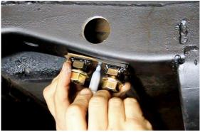
Figure 57 - Framerail Nut Plate Location
