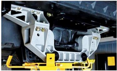
Figure 91 – Assemble the IRS Upper and Lower Cradle
