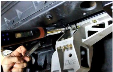
Figure 92 – Torque Upper Differential Bracket
