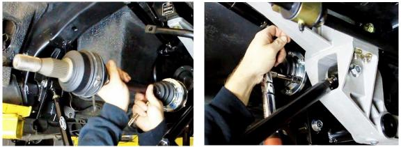
Figure 102 – Install Inner CV Joint to Stub Axle
