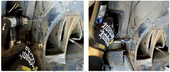
Figure 14 - Drill Trailing Link Holes
