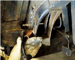
Figure 12 – Tack Weld Doubler Plate
