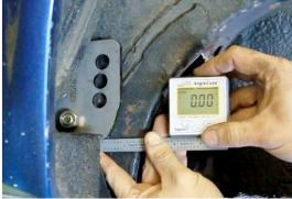
Figure 8 – Level Frame Doubler Plates
