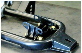
Figure 78 – Lower Differential Bracket Assembly Page 32 of 49
