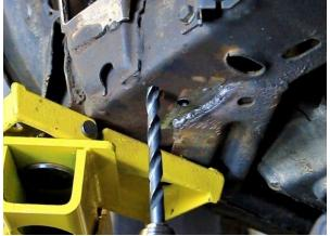
Figure 28 – Drill Trailing Arm Bracket Mounting Locations
