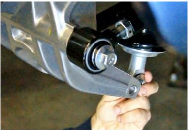
Figure 112 - Install Lower Shock Bolt & Tapered Spacers
