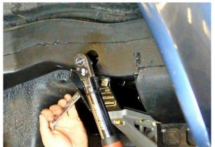
Figure 86 – Torque Inner Frame Rail Fasteners
