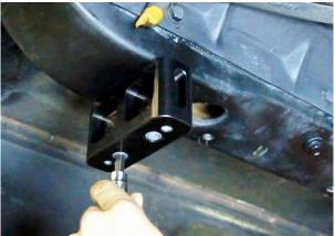
Figure 66 – Install Sway Bracket Spacer
