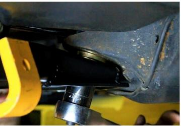
Figure 90 - Torque Lower Differential Mount
