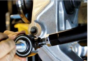
Figure 106 – Install Toe Links Page 42 of 49
