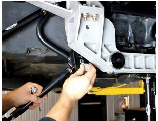
Figure 98 – Install Lower Lateral Links
