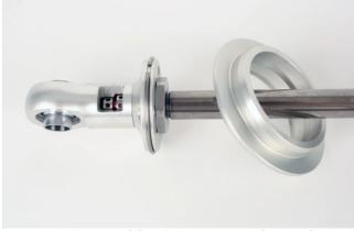
Figure 108 – Removing the Spring Seat
