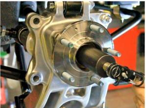
Figure 113 – Torque Outer CV Joint
