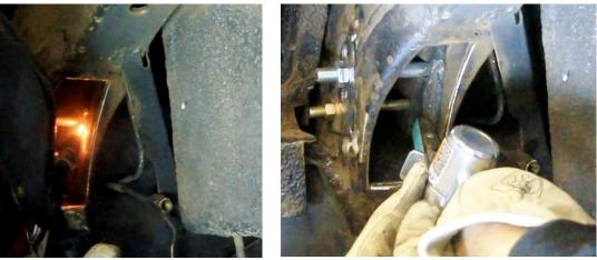
Figure 20 – Weld Inner Frame Rail
