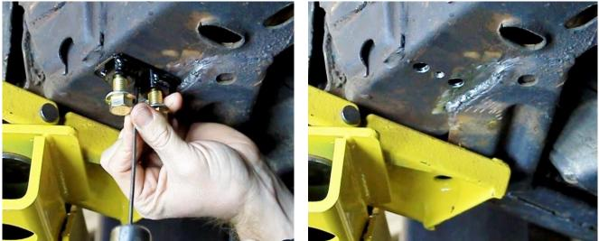
Figure 29 – Trailing Link Bracket Nut Plate
