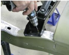
Figure 45 - Drill IRS Cradle Mount Locations
