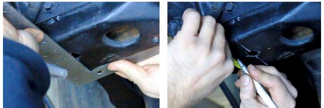
Figure 61 – Sway Bar Nut Plate Location
