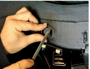
Figure 114 – Install Recessed Plug
