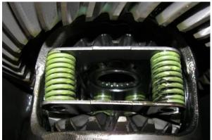
Figure 73 – Remove Stock Stub Axles
