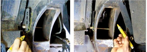
Figure 9 – Trace Outer and Inner Frame Doubler Plates
