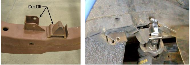
Figure 4 – Remove Frame Bumper and Upper Shock Mount Brackets
