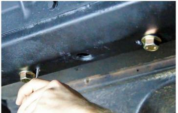
Figure 37 – Straighten Nut Plate & Clean Threads
