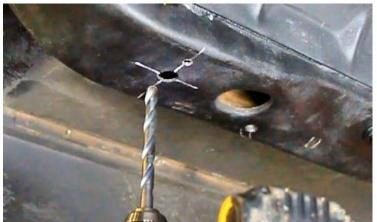
Figure 63 - Drill Sway Bar Nut Plate Location
