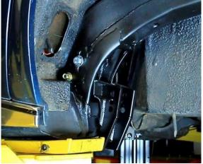
Figure 32 - Install Trailing Link Bracket
