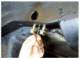
Figure 60 – Install Nut Plate Assemblies
