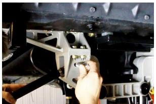
Figure 99 - Install Toe Link Assemblies
