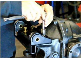
Figure 76 - Upper Differential Bracket Assembly
