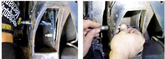
Figure 17 – Center Drill Inner Frame Rail
