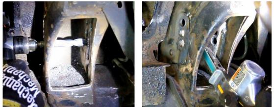
Figure 21 – Drill Upper & Lower Link Holes
