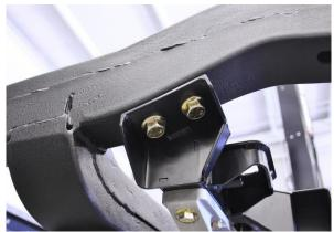
Figure 80 - Install Upper Cradle Assembly to Frame
