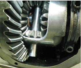
Figure 75 – Install Cross Shaft Page 31 of 49
