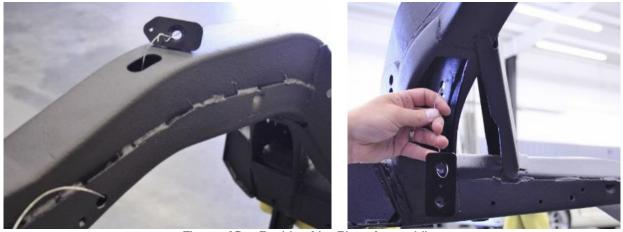
Figure 48 – Position Nut Plate Assemblies
