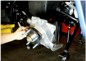
Figure 103 - Install Rear Upright to Outer CV Joint
