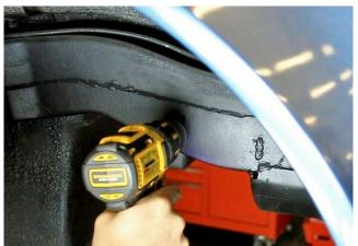
Figure 54 – Drill through Frame Rail
