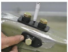
Figure 46 - Framerail Nut Plate Location
