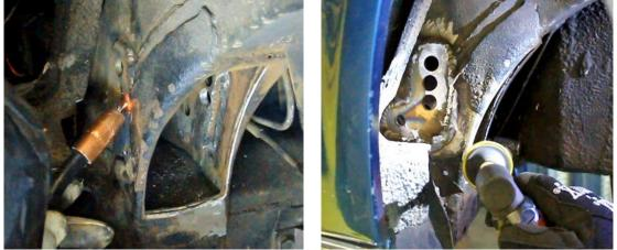
Figure 22 – Finish Weld Doubler Plates
