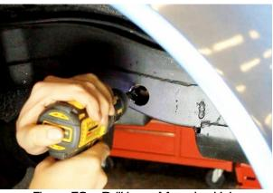
Figure 56 – Drill Inner Mounting Hole
