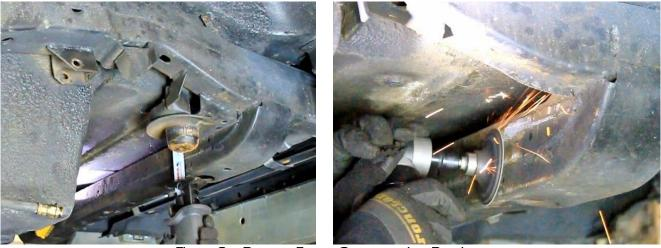
Figure 3 – Remove Frame Crossmember Brackets
