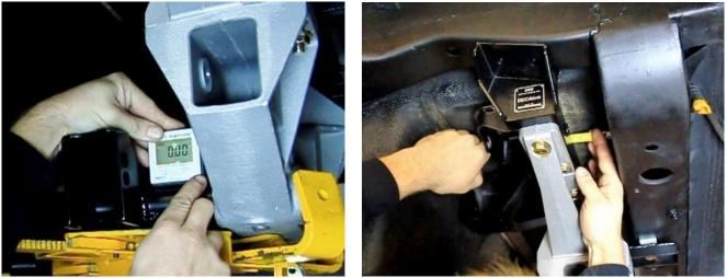
Figure 42 – Level IRS Cradle to the Frame
