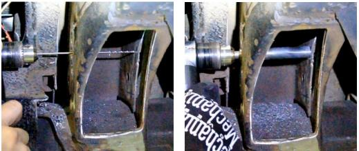
Figure 18 – Drill Inner Frame Rail
