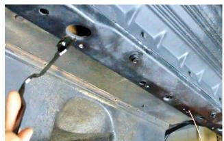
Figure 36 - Bend Crossmember Nut Plate
