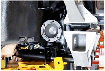
Figure 88 - Install 5/8"-18 Hardware
