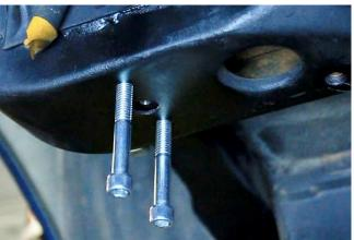
Figure 64 – Locate Sway Bar Nut Plate
