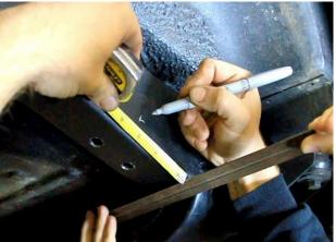
Figure 53 - Locate Access Holes
