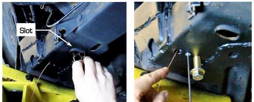
Figure 31 – Install Trailing Link Bracket Nut Plate
