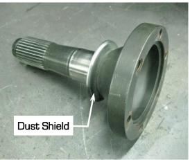
Figure 67 – Stub Axle Shafts
