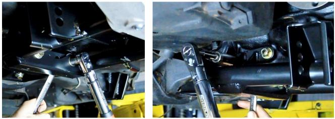
Figure 93 – Torque Lower Differential Bracket
