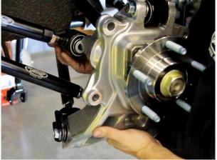
Figure 105 - Install Upper & Lower Trailing Links
