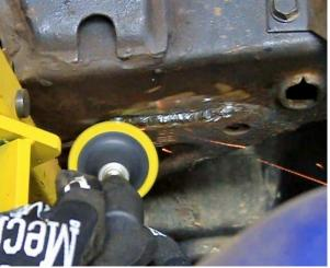
Figure 27 - Weld & Grind Gusset
