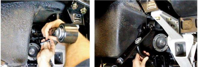
Figure 97 - Install Upper Lateral Link & Tie Braces
