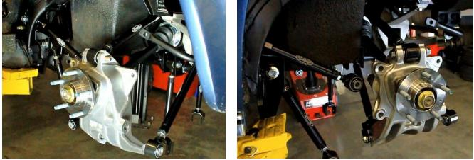
Figure 104 – Attach Lateral Links to Upright
