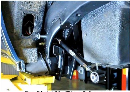
Figure 94 - Install the IRS Lower Trailing Links
