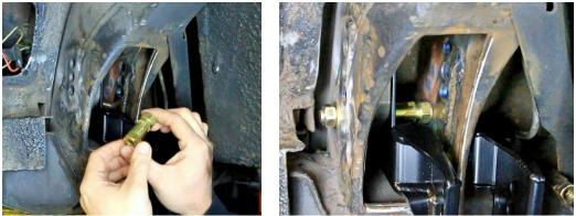
Figure 23 – Trailing Link Bracket
