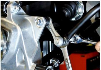
Figure 107 – Install Sway Bar End Link Assemblies
