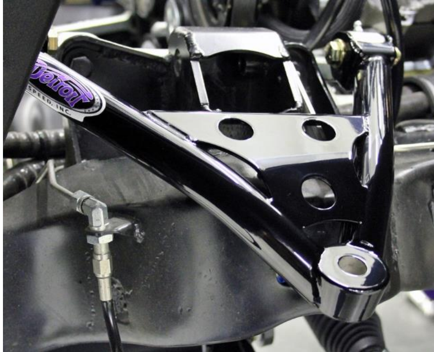
Figure 13 - Driver Side Upper Control Arm
