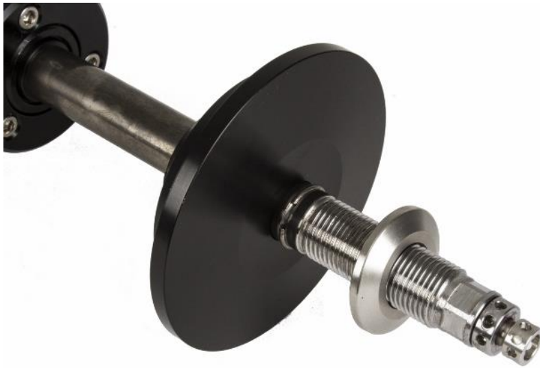
Figure 25 - Retaining Ring Installed
