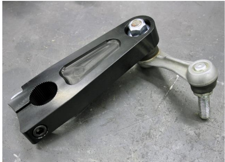
Figure 19 – Install Endlinks to the Sway Bar Arms
