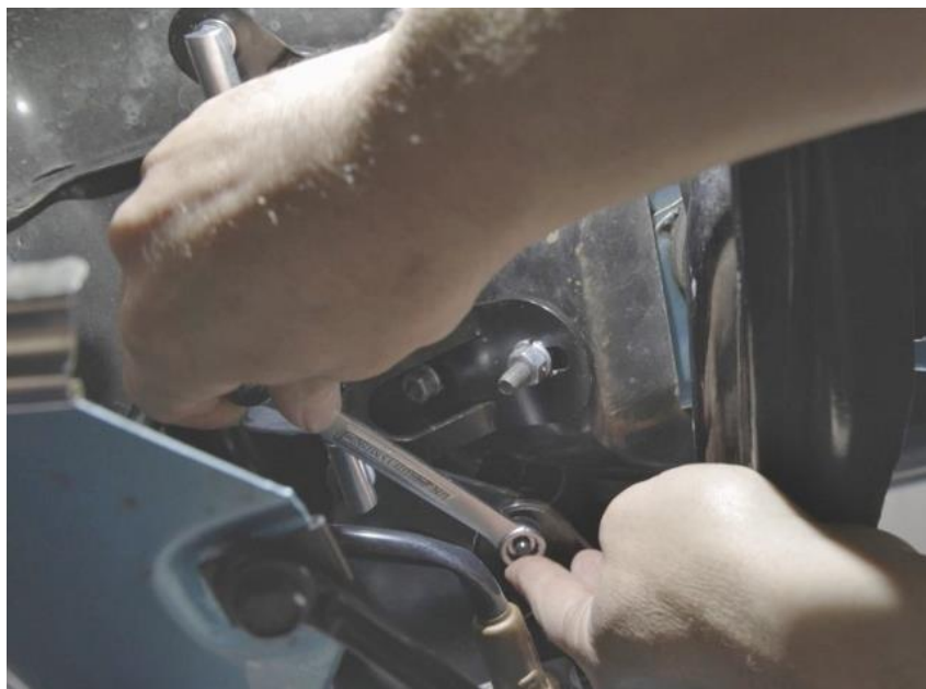
Figure 38 – Adjust Bell Crank Fastener
