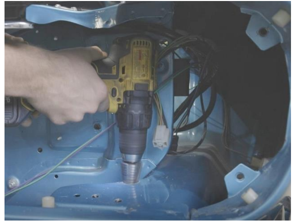
Figure 18 – Drill Template Holes
