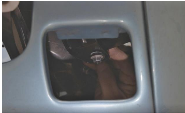
Figure 21 – Install Bell Crank Fasteners
