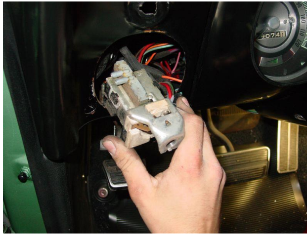
Figure 8 - Accessing the Headlamp Switch
