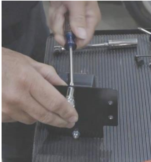
Figure 5 – Remove Wiper Module from Mounting Plate
