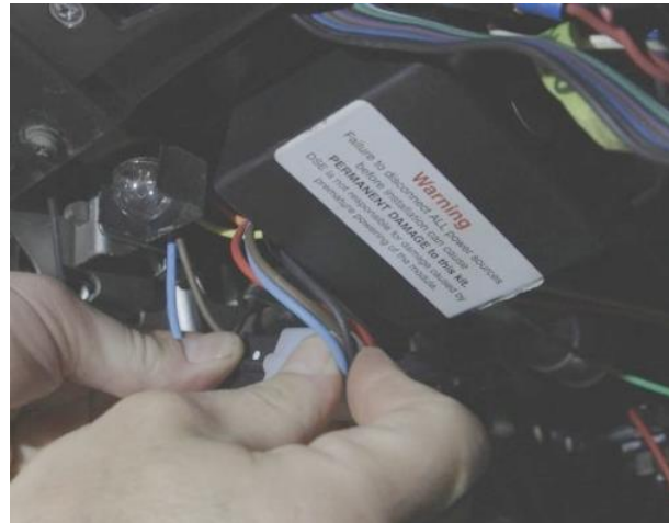
Figure 35 – Connect Module to Harness
