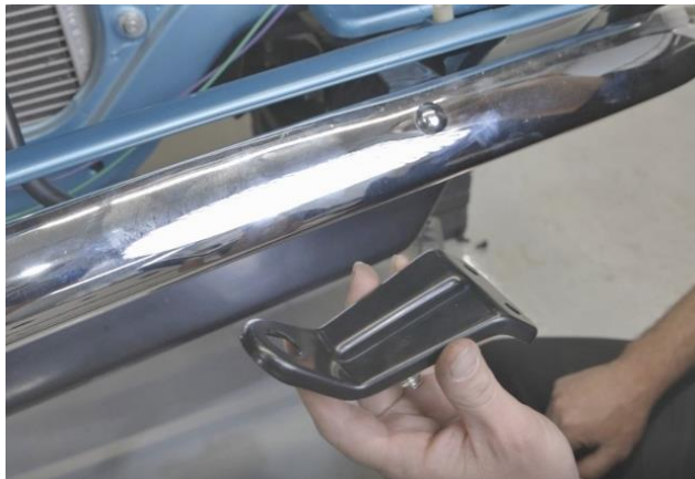
Figure 19 – Install Bell Crank Support Bracket
