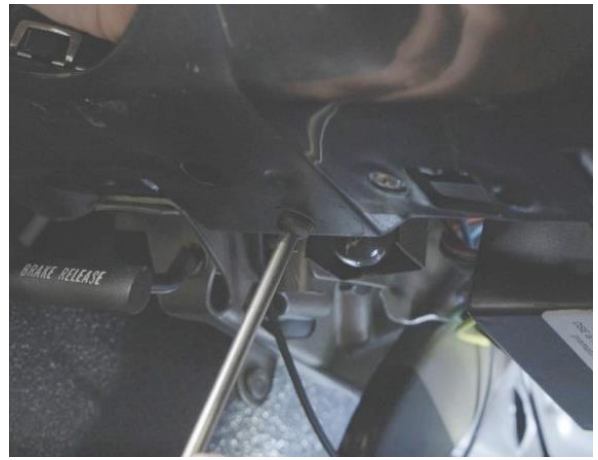
Figure 34 – Connect Ground Wire
