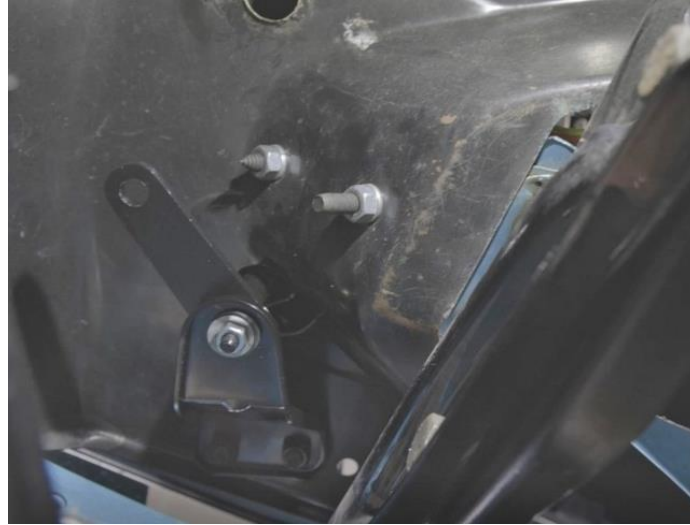
Figure 24 – Remove Core Support Fasteners
