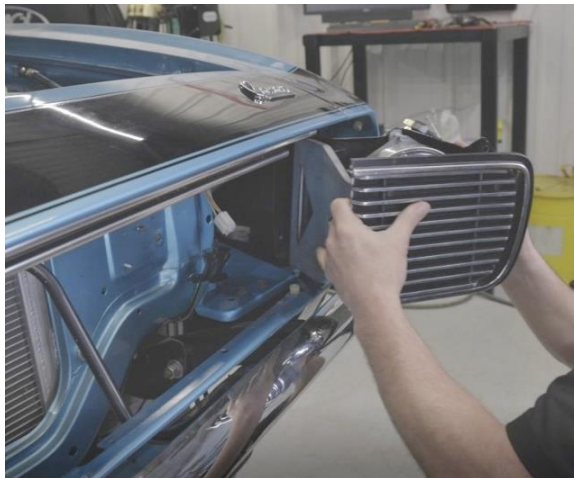
Figure 22 – Re-install Headlight Door Assembly
