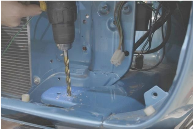
Figure 18 – Drill Template Holes
