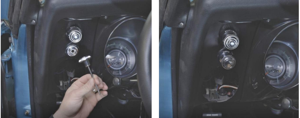
Figure 42 – Re-install Headlight Knob
