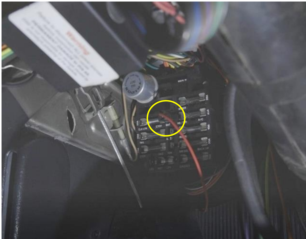
Figure 33 – Attach 12V Constant Power Source
