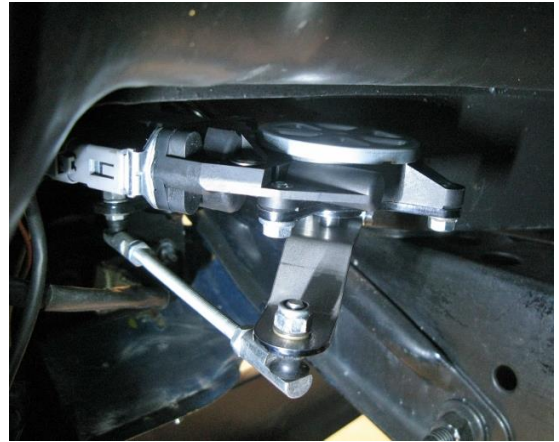
Figure 29 - Connect Actuator Linkage
