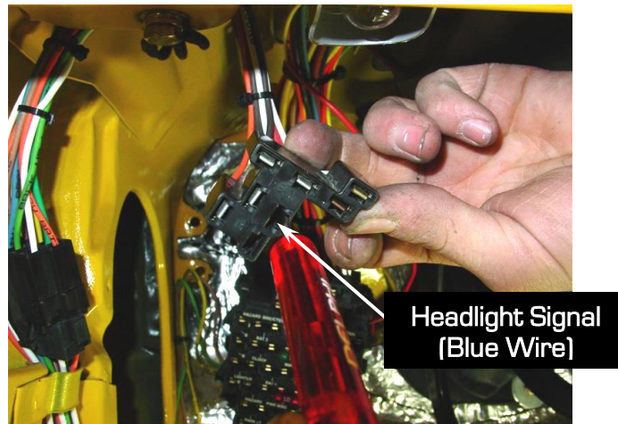
Figure 9 - Locating the Blue Wire
