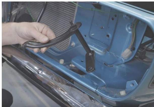
Figure 20 – Position Bell Crank
