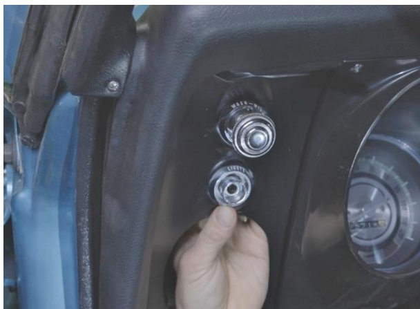
Figure 41 - Re-install Headlight Bexel and Switch Nut
