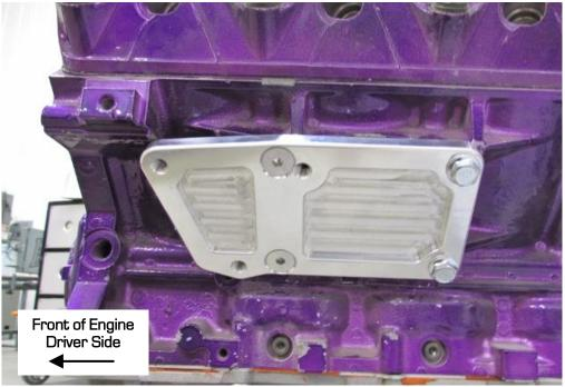
Figure 1 - Install Adapter Plate
