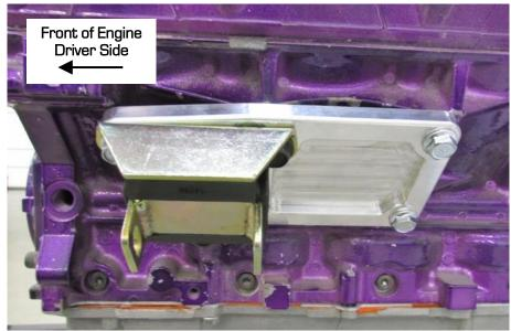
Figure 2 - Install Engine Mount
