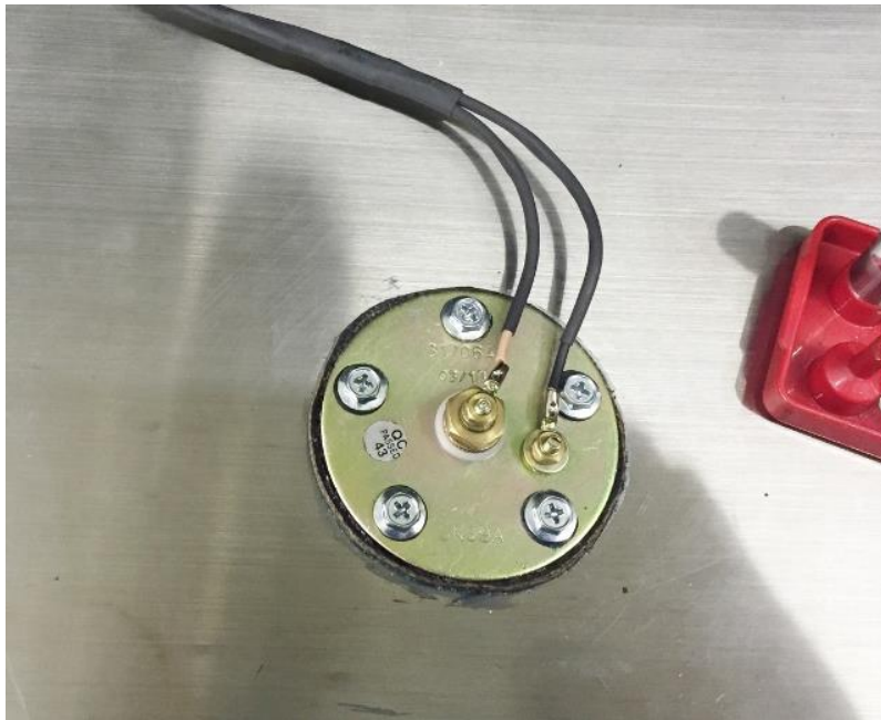
Figure 4 – Sending Unit and Fuel Pump Opening
