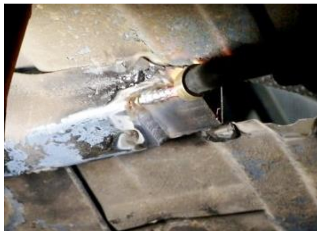
Figure 43 - Weld Back of Connector
