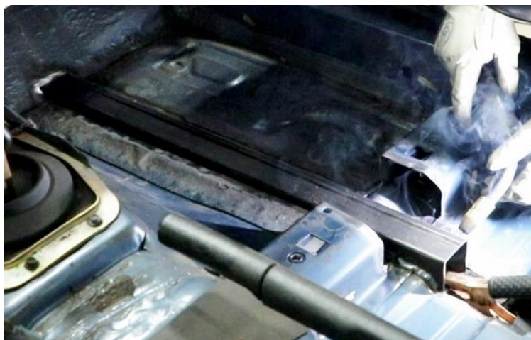
Figure 44 - Weld Sides of Connector
