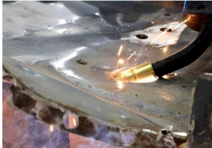
Figure 49 – Tack Weld Torque Box
