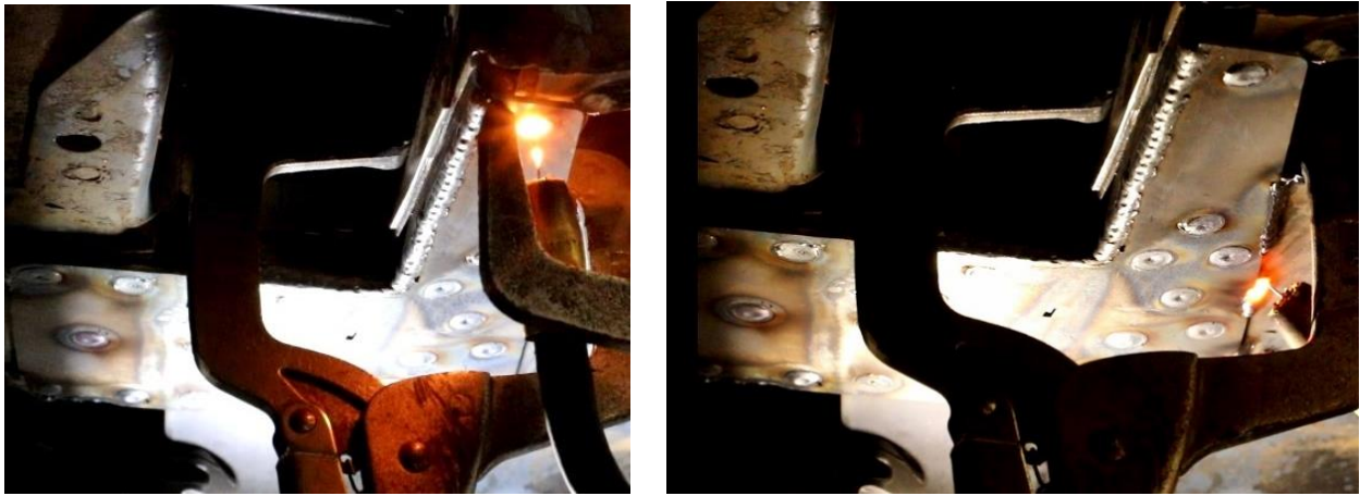
Figure 51 – Plug Weld Torque Box
