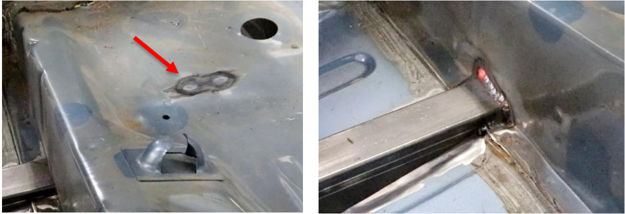
Figure 57 - Weld Seat Riser to Connector
