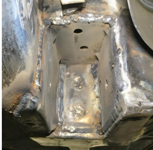
Figure 54 - Weld Factory Sheet Metal
