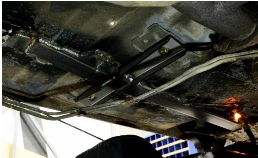
Figure 59 – Finish Weld Rear Connector
