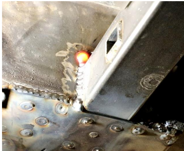
Figure 52 – Weld Rear Connector
