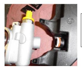
With the reservoir removed from the pump, place the O-ring on the reservoir stem followed by the Teflon spacer. Re-install the reservoir on the pump.
