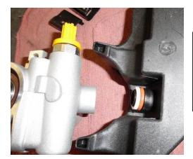
With the reservoir removed from the pump, place the O-ring on the reservoir stem followed by the Teflon spacer. Re-install the reservoir on the pump.
