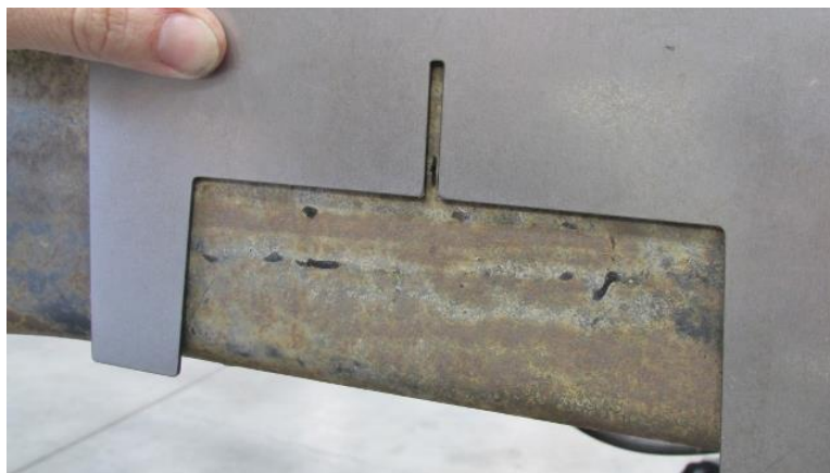
Figure 4 - Frame Notch Template
