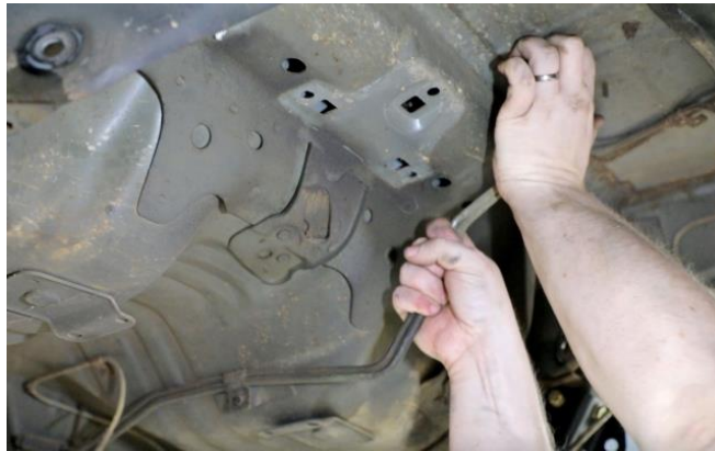
Figure 21 - Bend Fuel Lines
