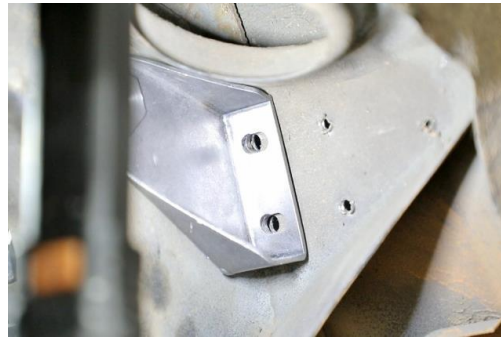
Figure 66 - Drill Floor Pan Holes
