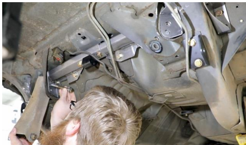
Figure 86 - Re-install Upper Trailing Links
