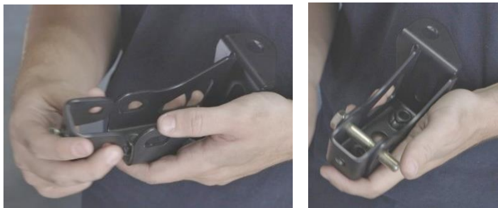
Figure 53 - Assemble Sway Bar Bracket
