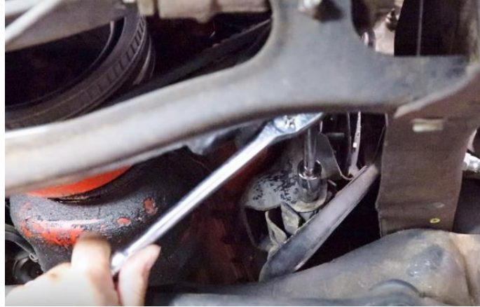
Figure 8 - Remove Engine Mount Hardware
