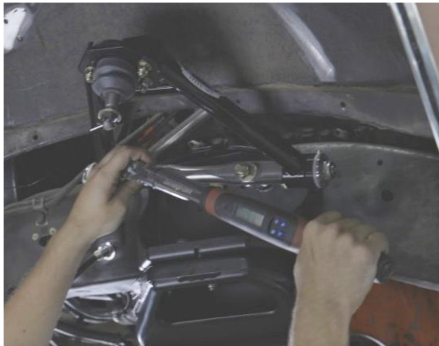
Figure 47 – Torque Upper Control Arms
