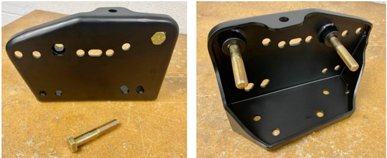
Figure 32 – Install Upper Control Arm Bolts
