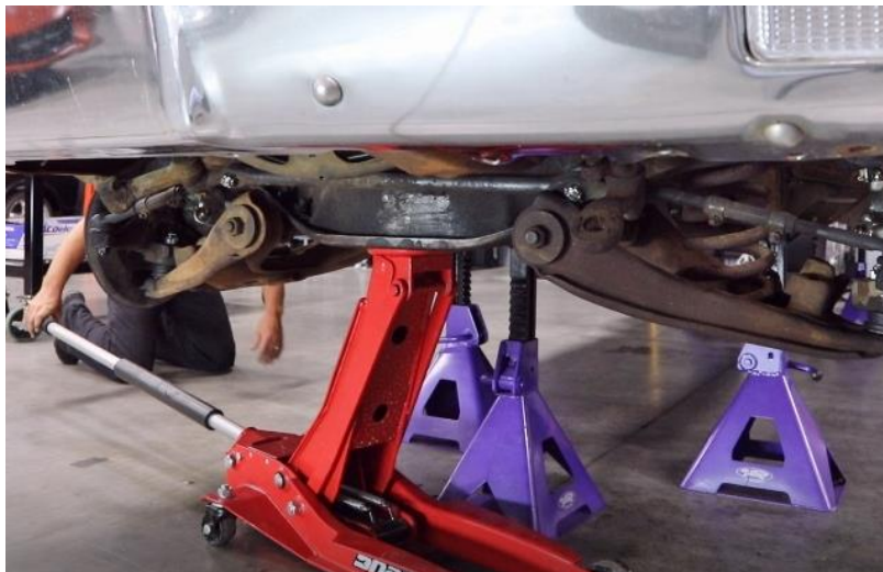
Figure 16 - Prepare to Remove the Cradle
