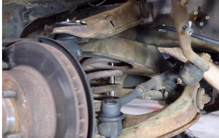
Figure 14 - Remove Cradle Hardware
