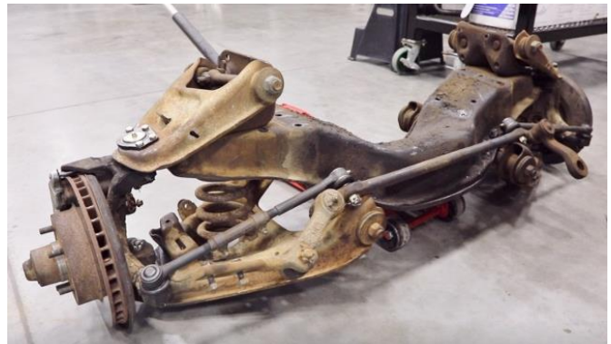
Figure 18 – Remove the Factory Cradle
