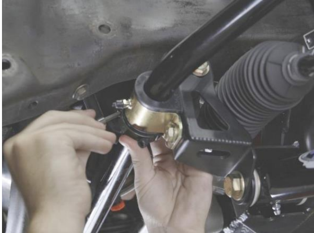
Figure 91 – Install Split Lock Collars
