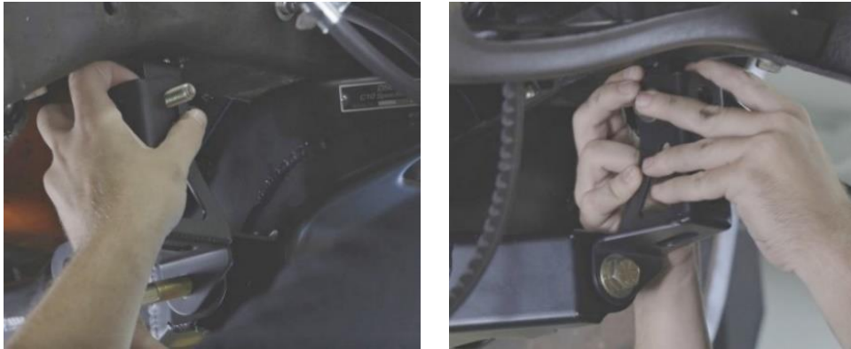
Figure 54 - Locate Sway Bar Bracket
