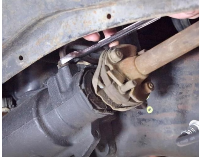
Figure 20 - Remove Power Steering Lines
