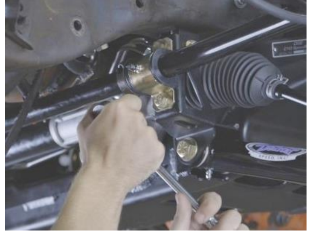
Figure 91 – Install Split Lock Collars
