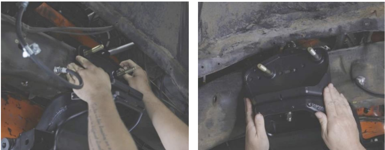
Figure 33 – Locate Upper Control Arm Brackets
