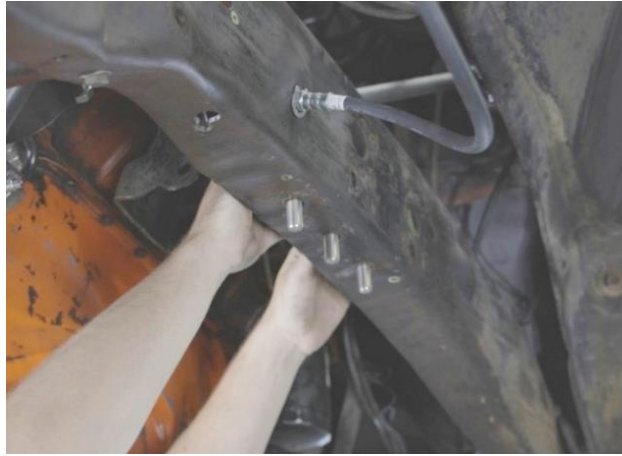
Figure 25 - Locate Bolts in Frame Rails
