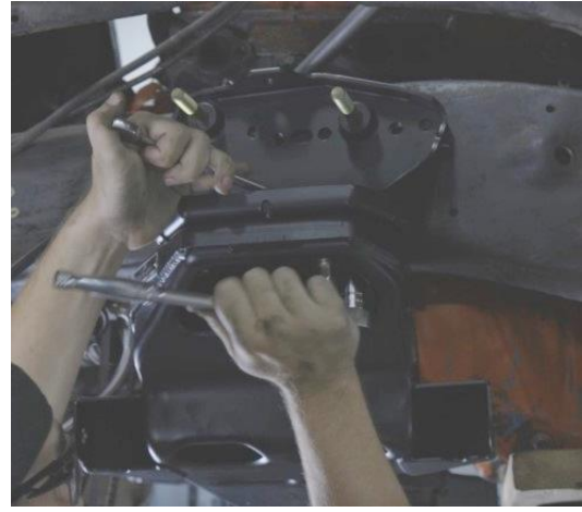
Figure 34 - Loosley Install Upper Control Arm Brackets
