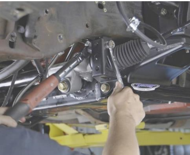
Figure 70 - Torque Lower Control Arm
