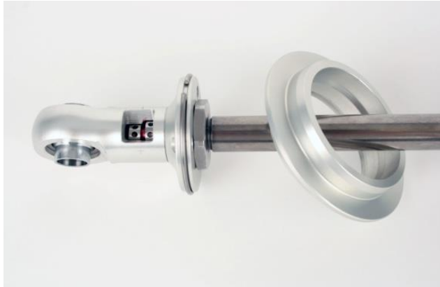
Figure 78 – Remove Upper Spring Seat
