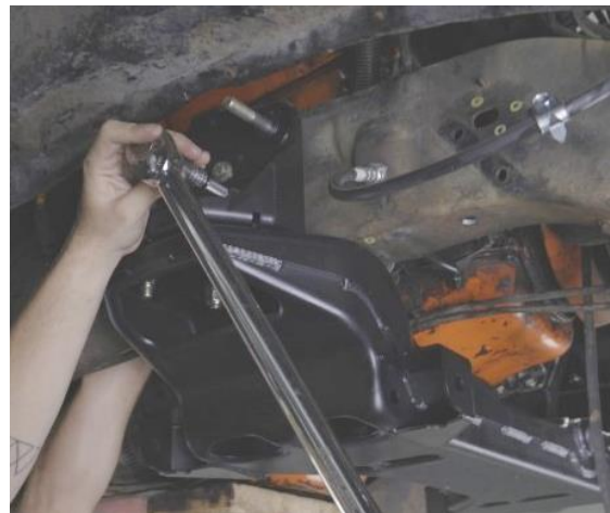
Figure 44 - Torque Cradle Hardware
