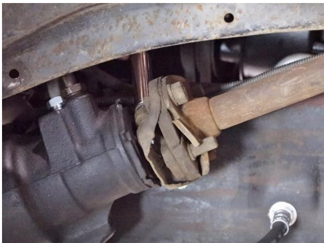
Figure 19 – Remove the Rag Joint
