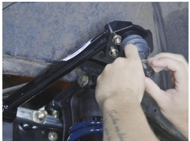
Figure 93 – Remove Ball Joint Hardware
