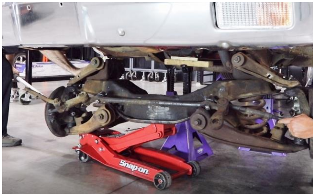
Figure 18 – Remove the Factory Cradle
