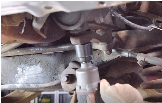
Figure 7 - Remove Pitman Arm
