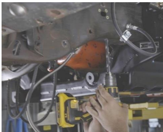
Figure 56 - Drill Sway Bar Bracket Mounting Hole
