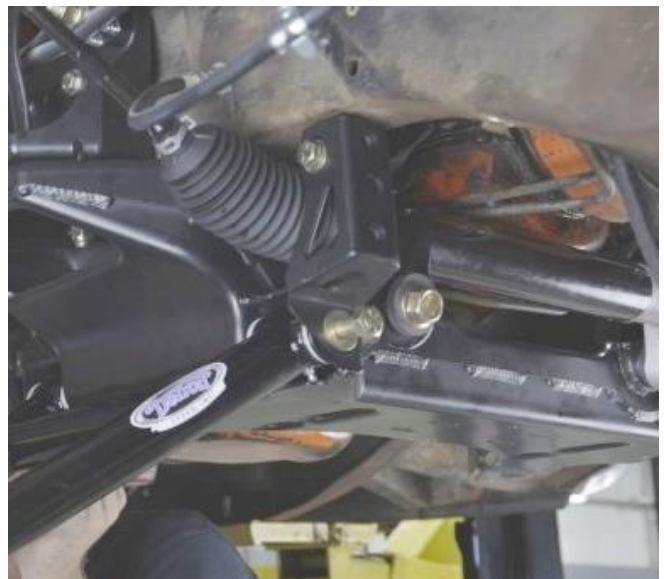
Figure 68 – Install Front Lower Control Arm Hardware
