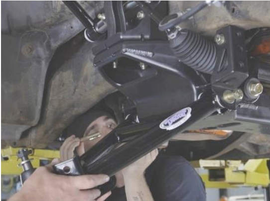
Figure 69 - Tighten Lower Control Arm
