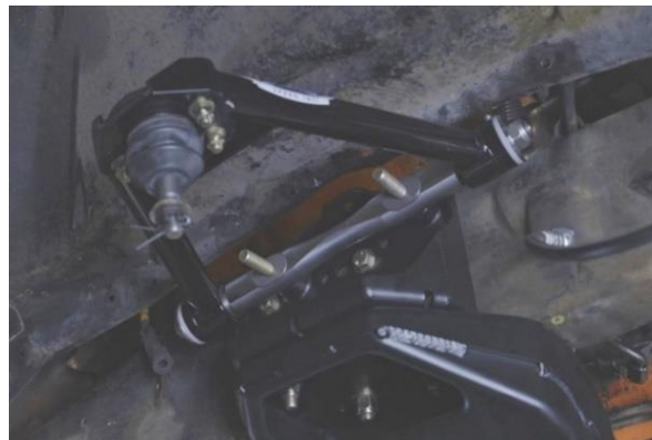
Figure 45 - Install Upper Control Arms
