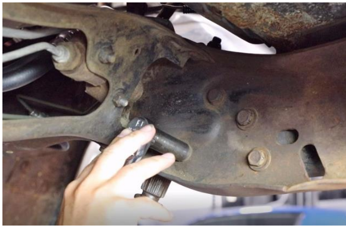
Figure 21 - Loosen Steering Gear Bolts
