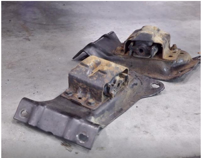
Figure 12 – Remove Engine Mount Brackets
