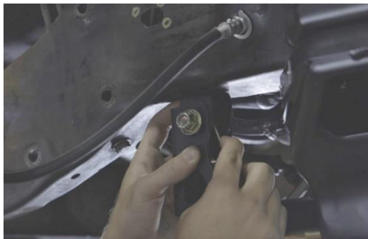
Figure 55 - Scribe Sway Bar Bracket Mounting Hole
