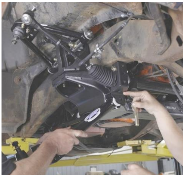
Figure 68 – Install Front Lower Control Arm Hardware
