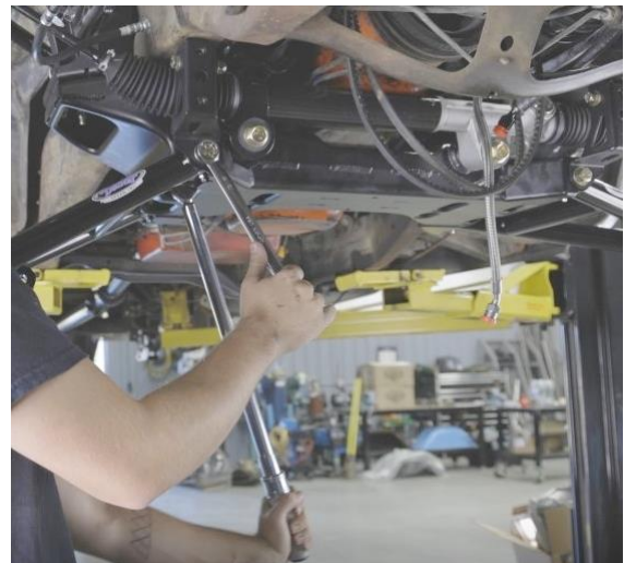
Figure 70 - Torque Lower Control Arm
