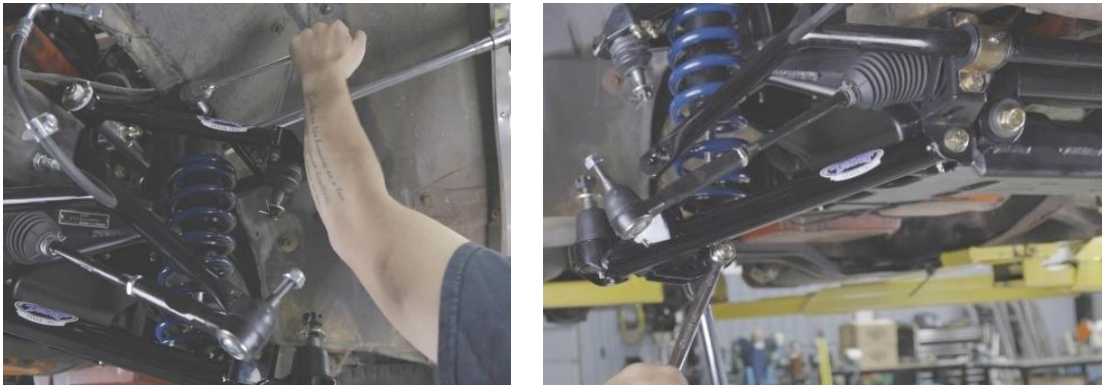
Figure 86 - Torque Shock Hardware
