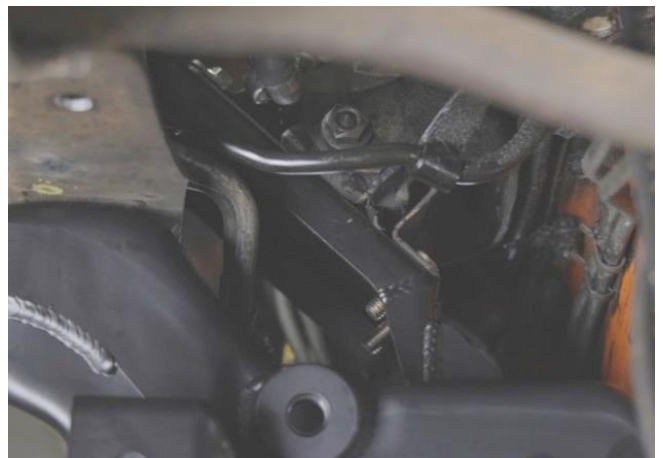
Figure 42 – Install Engine to Brackets
