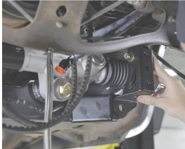
Figure 66 – Install Sway Bar Bracket Hardware
