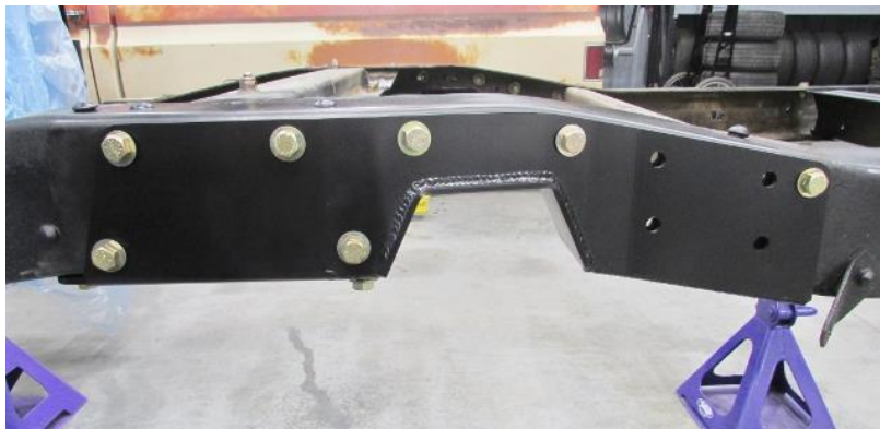
Figure 14 - Install (LH, Driver Side) Frame Rail Notch Bracket
