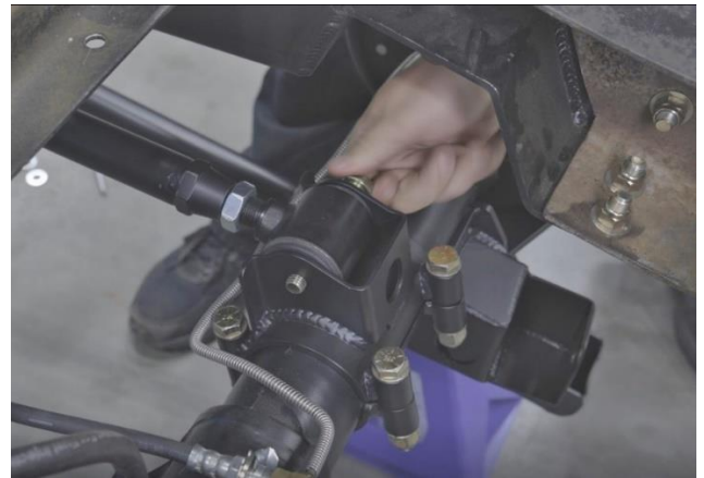
Figure 19 – Install Swivel Links at Axle
