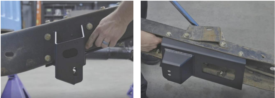
Figure 8 - Install Chassis Bracket Assembly
