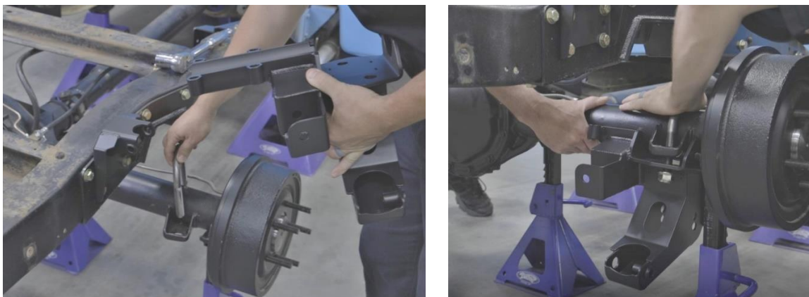
Figure 14 - Install Track Bar Bracket
