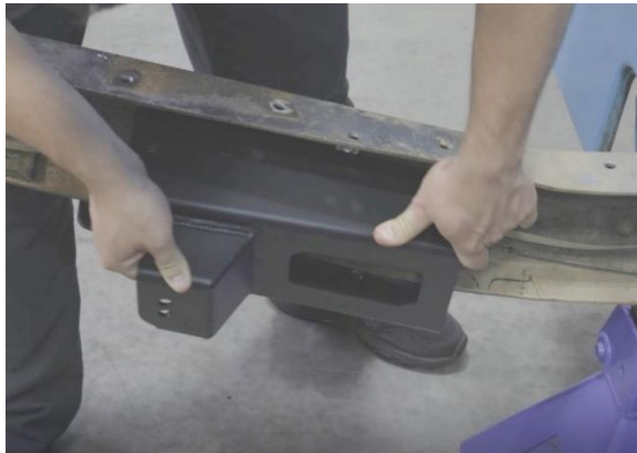
Figure 5 – Locate Chassis Bracket Assembly
