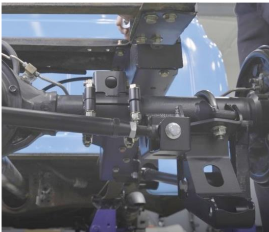
Figure 20 – Install Track Bar at Axle
