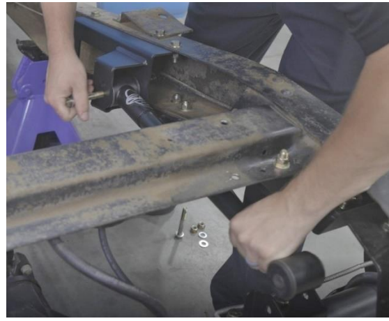
Figure 18 – Install Swivel Links at Chassis
