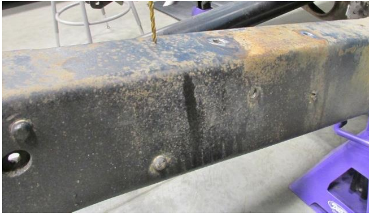
Figure 4 – Drill Bracket Mounting Holes
