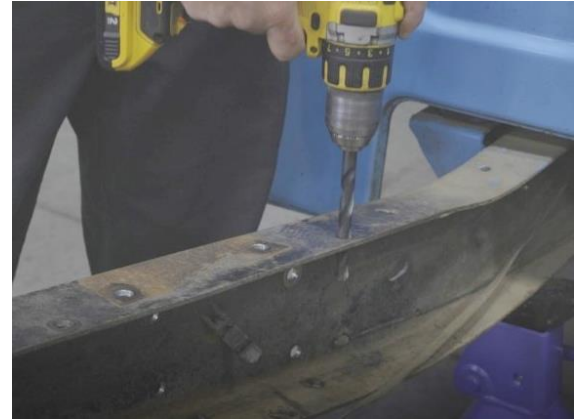
Figure 4 – Drill Bracket Mounting Holes
