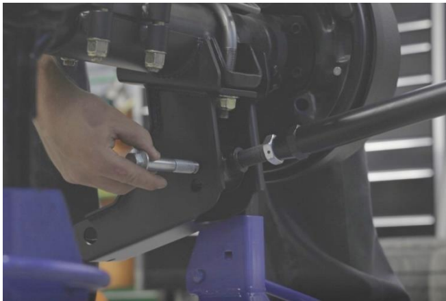
Figure 19 – Install Swivel Links at Axle
