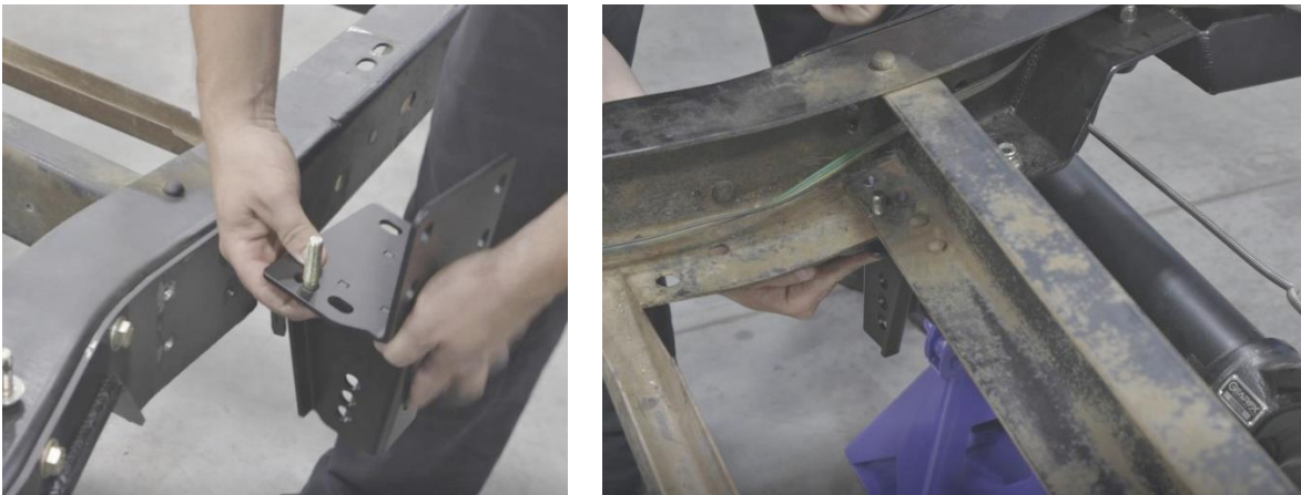
Figure 9 - Mount Track Bar Bracket
