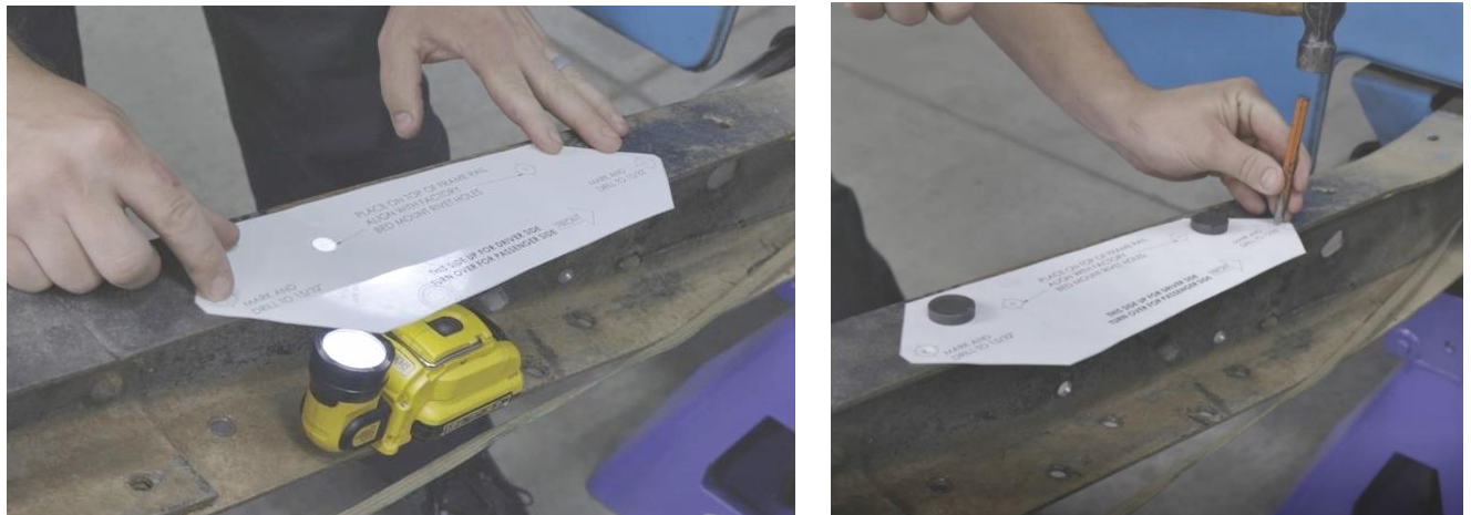
Figure 3 - Transfer Punch Top Framerrail
