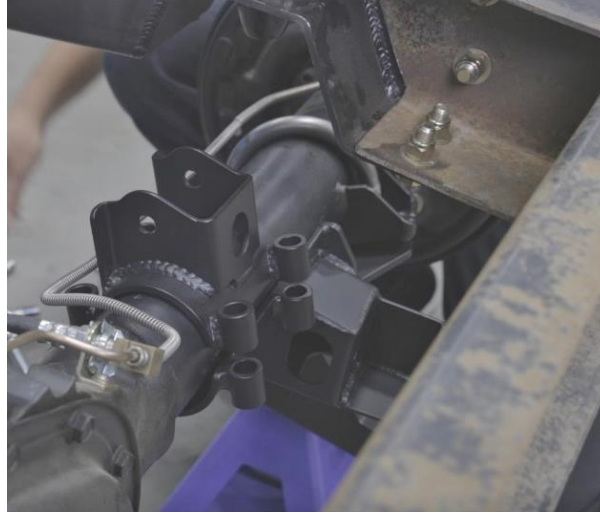
Figure 15 - Locate Upper Axle Bracket
