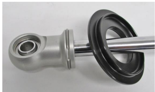
Figure 28 - Install Spring Perch
