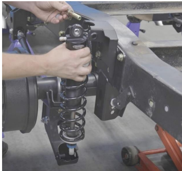
Figure 31 – Install Shock in Upper Shock Mount
