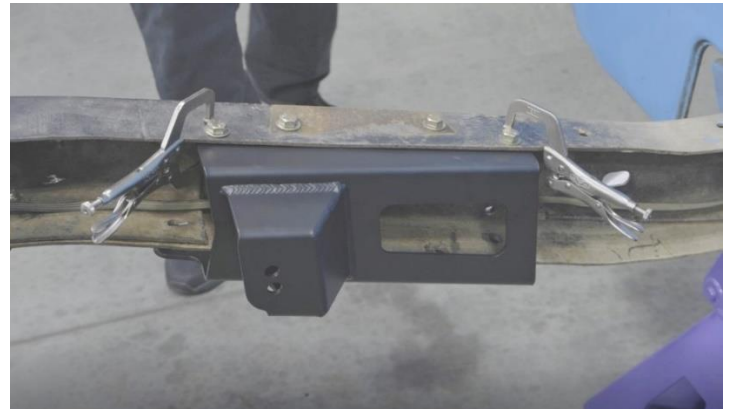
Figure 5 – Locate Chassis Bracket Assembly
