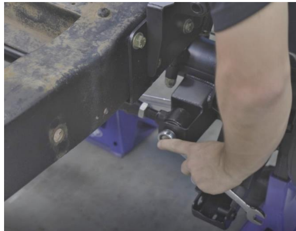
Figure 20 – Install Track Bar at Axle
