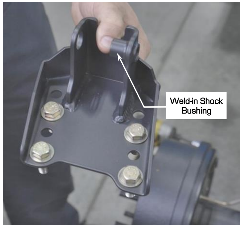
Figure 11 - Locate Upper Shock Mount
