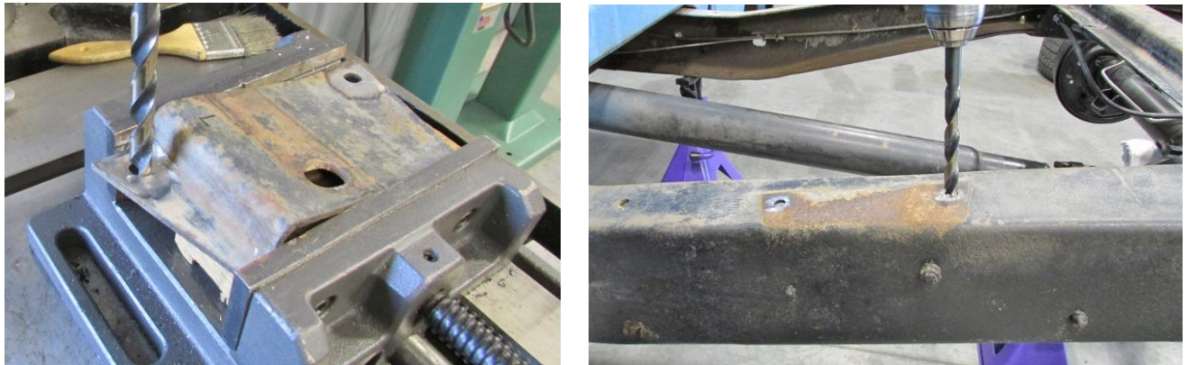
Figure 2 - Drill Out Brackets & Frame Rails
