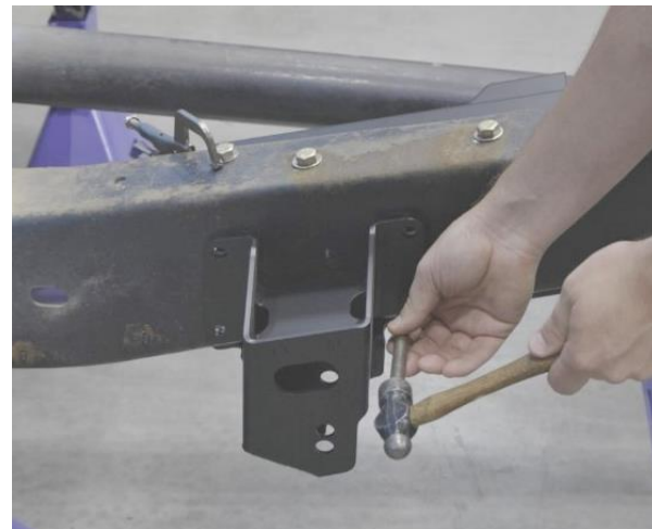
Figure 6 – Transfer Punch Outside Frameraill
