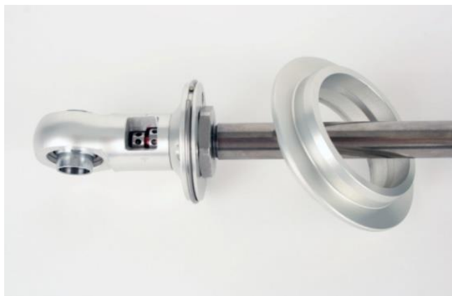
Figure 29 – Remove Upper Spring Seat
