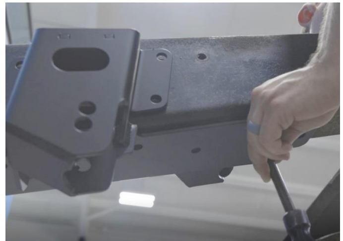
Figure 6 – Transfer Punch Outside Frameraill
