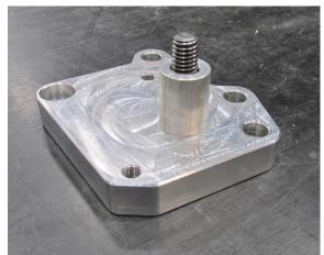
Figure 3 - Install Socket Head Bolt & Spacer
