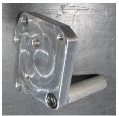
Figure 6 - Install Socket Head Bolt & Spacer
