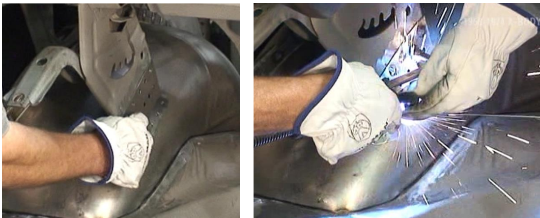
Figure 32 – Fabricate and Weld the Decklid Support
