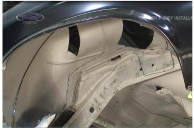
Figure 15 – Remove the Seat Brace
