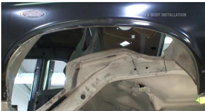
Figure 16 – Stock Inner Tub Removed
