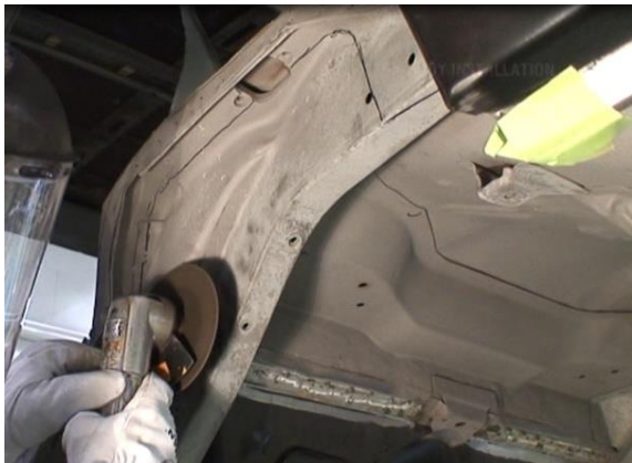
Figure 17 – Cutting along the Framerrail
