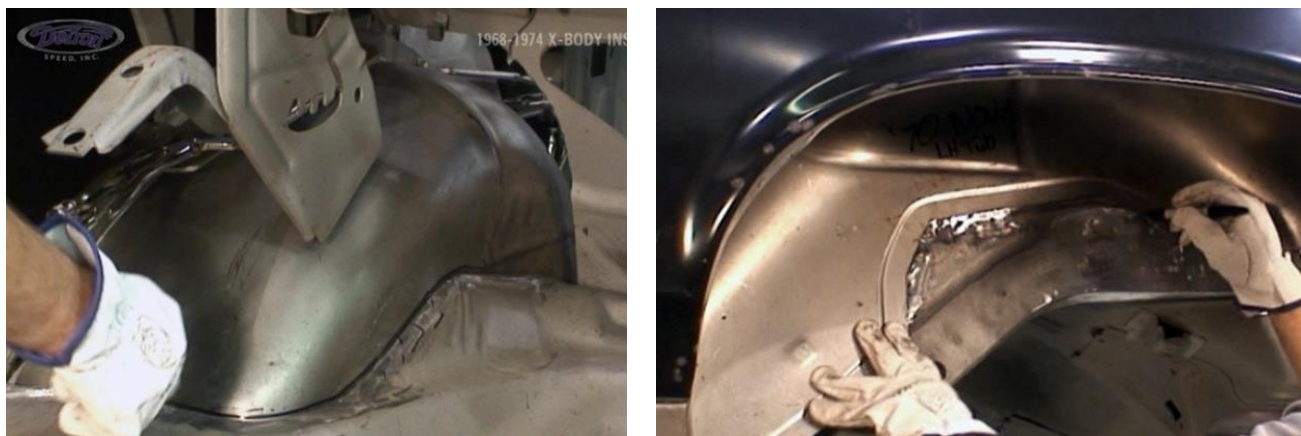
Figure 26 - Mark the Mini-Tub
