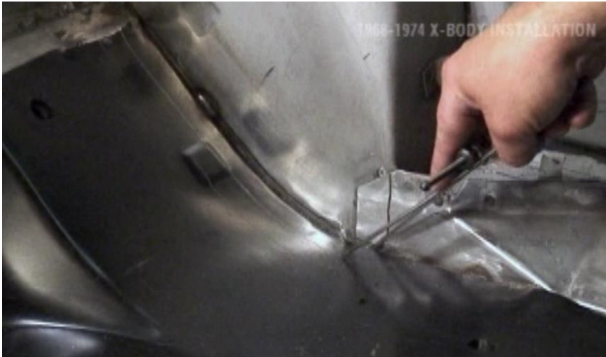
Figure 4 - Mark the Flange Bend Line
