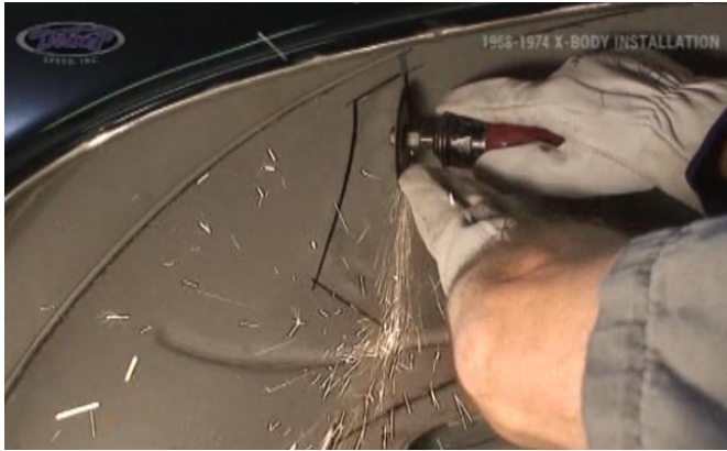
Figure 15 – Remove the Seat Brace
