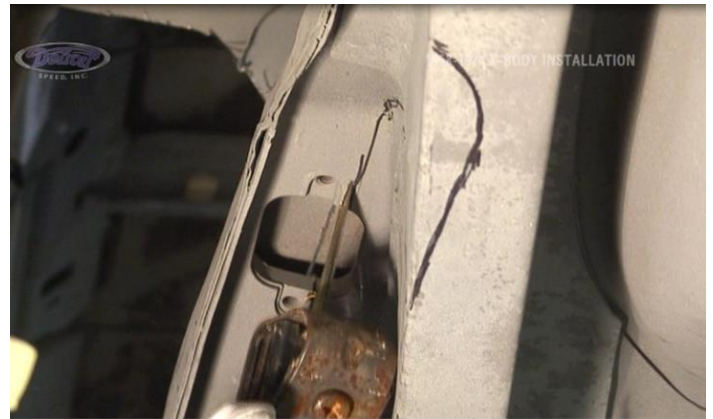
Figure 17 – Cutting along the Framerrail
