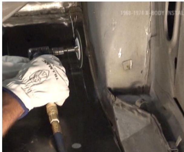
Figure 14 - Cut 1-1/4" Marked Lines
