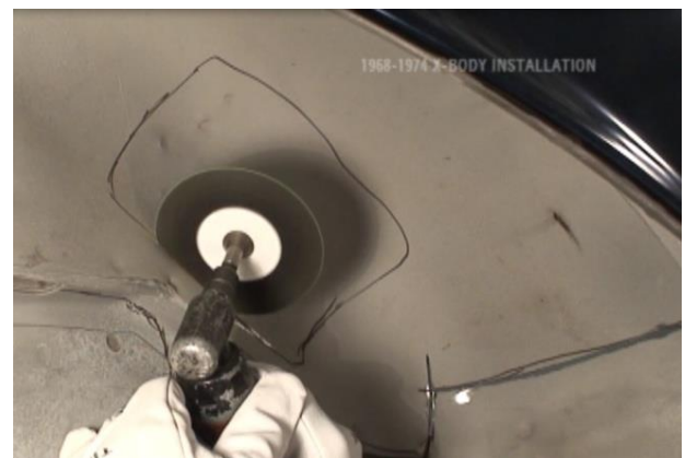
Figure 11 - Mark the Trunk Mounts
