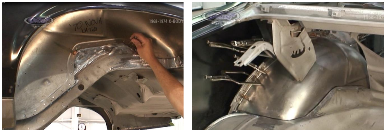
Figure 28 - Secure the Mini-Tub for Welding
