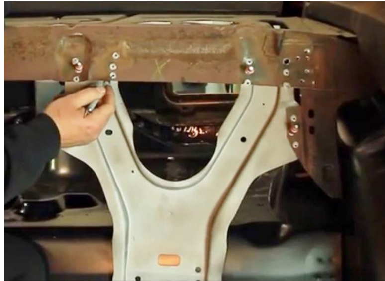
Figure 9 - Drill Out Spot Welds
