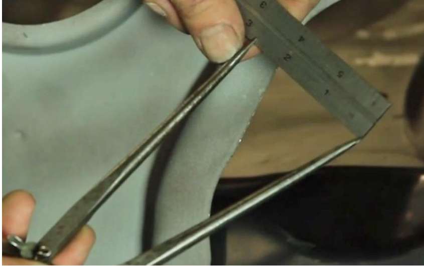
Figure 5 – Set Dividers and Transfer a 2-3/4" Scribe Line
