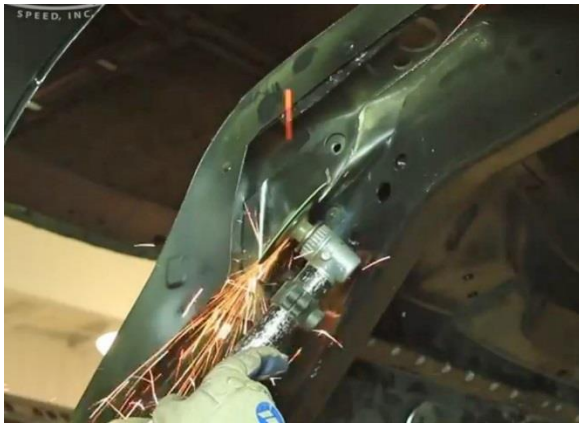
Figure 22 - Cutting the Frame Rail Reinforcement
