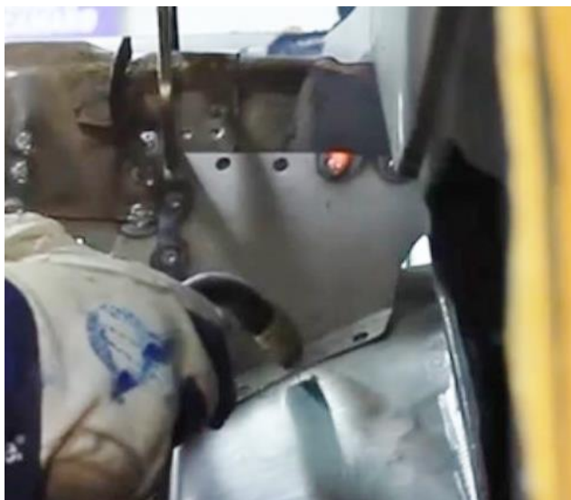
Figure 48 – Weld in Rear Seat Bracket Closeout
