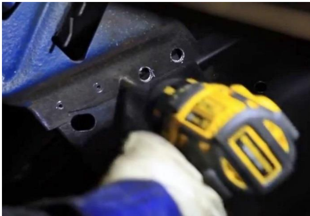
Figure 17 – Remove Decklid Reinforcement Bracket
