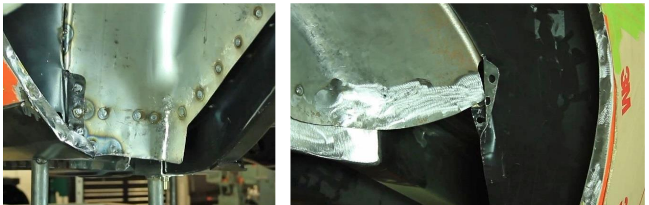
Figure 41 - Weld Outer Wheel Tub Flanges
