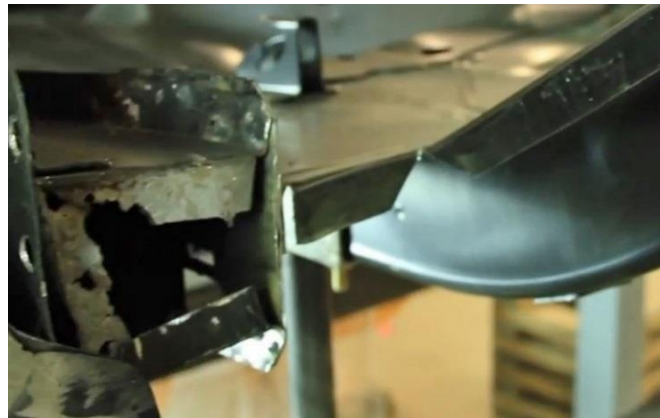
Figure 28 – Trim Rocker and Bend Fold Lines
