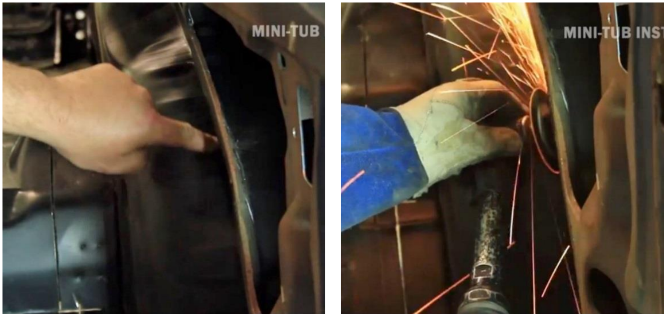
Figure 20 – Cut the Factory Bend Line
