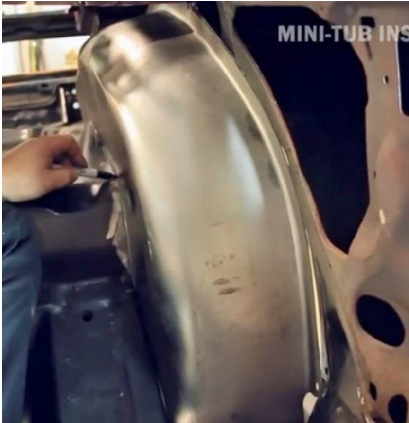
Figure 37 – Locate Trunk Floor Height
