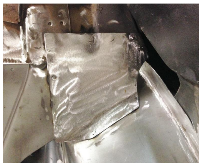
Figure 48 – Weld in Rear Seat Bracket Closeout
