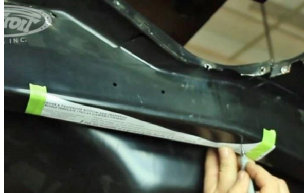
Figure 24 – Scribe Cut Line onto the Bottom Frame Rail
