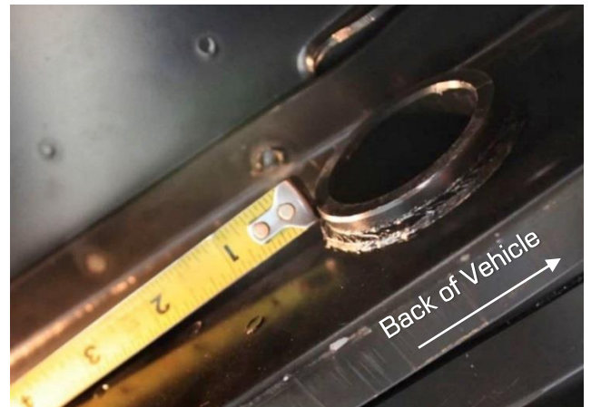
Figure 23 - Locate Bottom Frame Rail Cut Template
