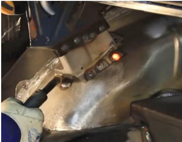
Figure 45 - Weld in Trunk Hinge Reinforcements.
