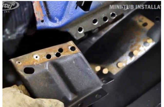
Figure 17 – Remove Decklid Reinforcement Bracket
