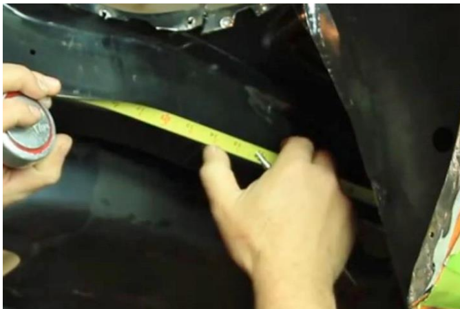
Figure 23 - Locate Bottom Frame Rail Cut Template
