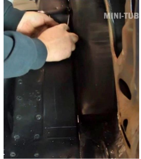
Figure 5 – Set Dividers and Transfer a 2-3/4" Scribe Line
