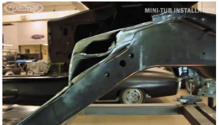
Figure 22 - Cutting the Frame Rail Reinforcement
