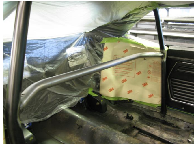
Figure 9 – (Finished Cross Brace)
