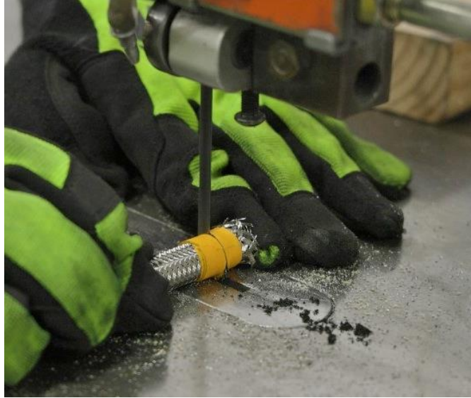
Figure 4 – Cut Hoses to Length
