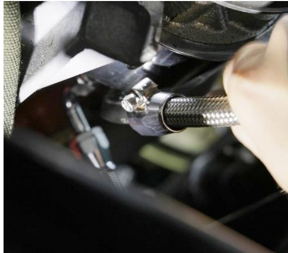
Figure 10 - Install Return Hose
