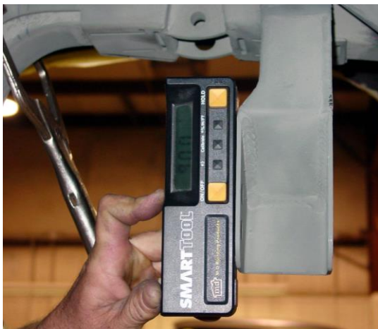
Figure 21 - Level the Track Bar Body Mount
