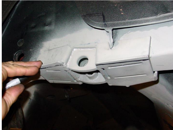
Figure 22 - Trim the Oversized Material
