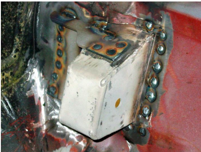
Figure 28 - Interior Floor Pan Doubler
