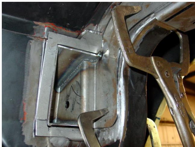
Figure 23 - Fit the Exterior Floor Pan Doubler
