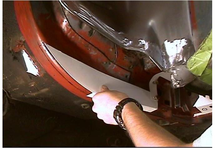
Figure 6 - Outboard Framerrail Template
