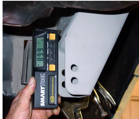
Figure 21 - Level the Track Bar Body Mount
