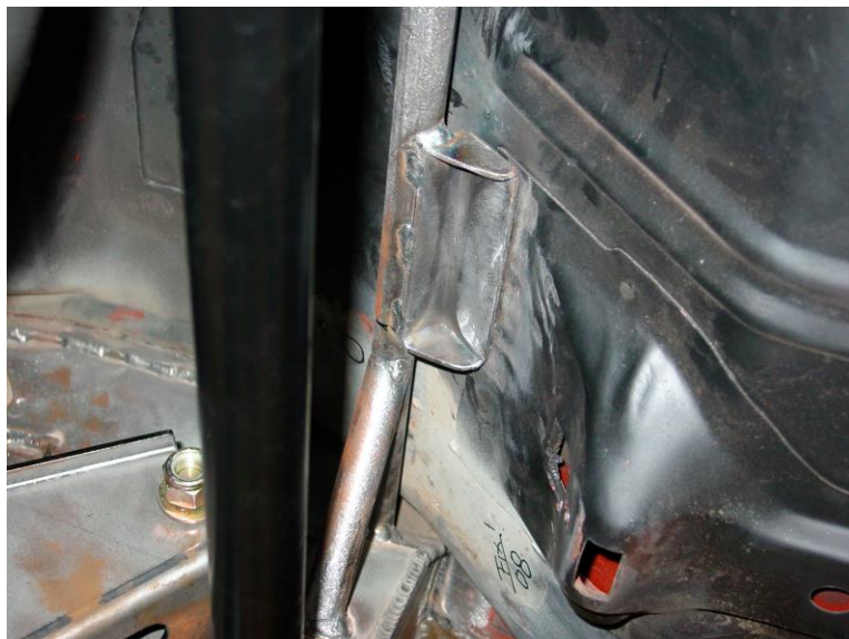
Figure 30 - Transverse Tube Bracket Installation
