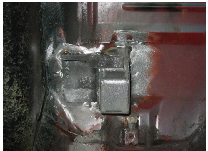
Figure 28 - Interior Floor Pan Doubler
