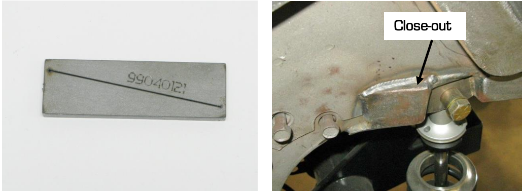
Figure 25 - Outboard Frame Rail Doubler Close-out
