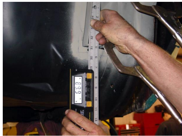
Figure 20 - Level the Upper Link Pocket
