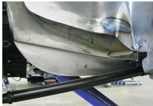
Figure 11 - Framerrail Fill Panel
