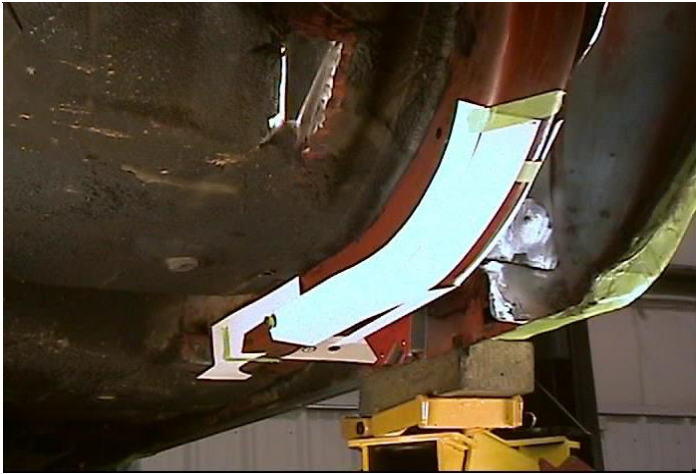
Figure 5 - Inboard Framerrail Template
