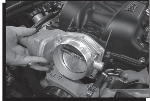
**Figure 12 Installing the Throttle Body.**
