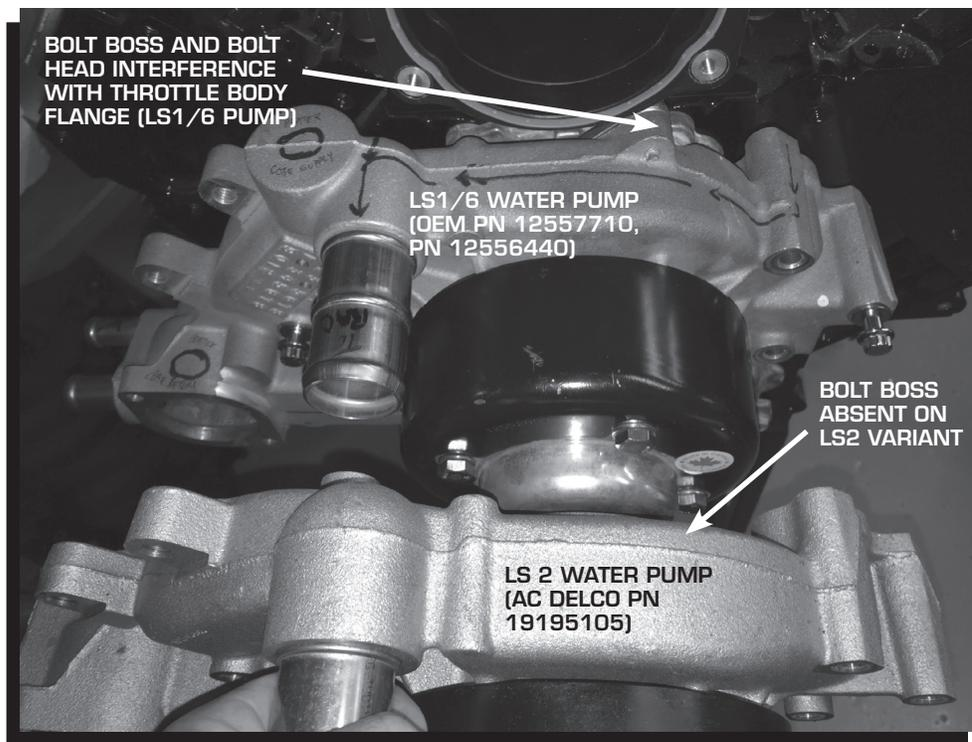
Figure 14 - LS1/6 and LS2 Water Pump Comparison
